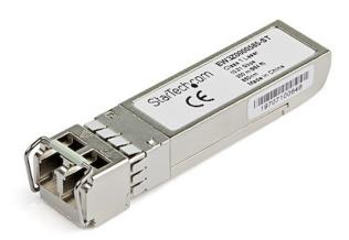
The EW3Z0000585-ST is a Citrix EW3Z0000585 compatible fiber transceiver module that has been designed, programmed and tested to work with Citrix brand switches and routers. It delivers dependable 10 GbE connectivity over fiber cable, for 10GBASE-SR compliant networks, with a maximum distance of up to 300 m (984 ft).
