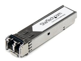
The JD094A-ST is an HPE JD094A compatible fiber transceiver module that has been designed, programmed and tested to work with HPE brand switches and routers. It delivers dependable 10 GbE connectivity over fiber cable, for 10GBASE-LR compliant networks, with a maximum distance of up to 10 km (6.2 mi).
