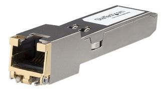
The JL563A-ST is a HPE JL563A compatible copper transceiver module that has been designed, programmed and tested to work with HPE brand switches and routers. It delivers dependable 10 GbE connectivity over copper cable, for 10/100/1000/10000 compliant networks, with a maximum distance of up to 30 m (98.4 ft).
