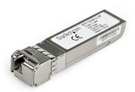
The SFP-10G-BXU-I-ST is a Cisco SFP-10G-BXU-I compatible upstream fiber SFP transceiver which pairs with StarTech.com's SFP-10G-BXD-I-ST. They are designed, programmed and tested to work with 10GBASE-BX compatible Cisco switches and routers. The SFP+ transceiver module supports a maximum distance of up to 10 km (6.2 mi) and delivers dependable 10 GbE connectivity over fiber cabling.
