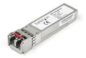
The SFP-10G-ER-ST is a Cisco SFP-10G-ER compatible fiber transceiver module that has been designed, programmed and tested to work with Cisco brand switches and routers. It delivers dependable 10 GbE connectivity over fiber cable, for 10GBASE-ER compliant networks, with a maximum distance of up to 40 km (24.8 mi).
