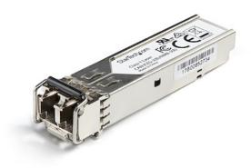
The SFP1GZXEMCST is a Dell EMC SFP-1G-ZX compatible fiber transceiver module that has been designed, programmed and tested to work with Dell EMC brand switches and routers. It delivers dependable 1 GbE connectivity over fiber cable, for 1000BASE-ZX compliant networks, with a maximum distance of up to 80 km (49.7 mi).
