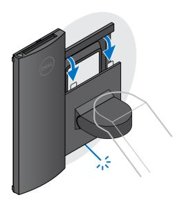
NOTE: To install the offset VESA mount on a Dell E-Series monitor, remove the VESA cover from the back of the monitor and secure the offset VESA mount along with the device to the monitor.
