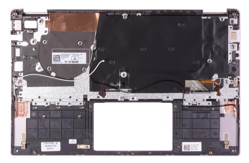
After performing the steps in the pre-requisites, we are left with the palm-rest and keyboard assembly.
