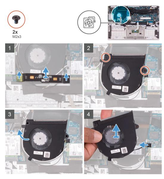
1 Disconnect the I/O-board cable from the system board and I/O board.
