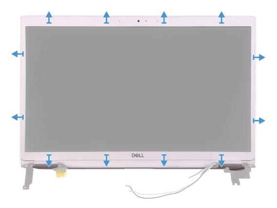
Align the display bezel with the display back-cover and antenna assembly, and gently snap the display bezel into place.
