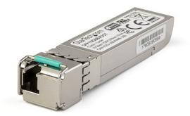
The SFP10GBX10DS is a Dell EMC SFP-10G-BX10-D compatible downstream fiber SFP transceiver which pairs with StarTech.com's SFP10GBX10US. They are designed, programmed and tested to work with 10GBASE-BX10 compatible Dell EMC switches and routers. The SFP+ transceiver module supports a maximum distance of up to 10 km (6.2 mi) and delivers dependable 10 GbE connectivity over fiber cabling.
