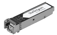
The SFPGE10KT5R3 is a Juniper SFPP-10GE-LR compatible fiber transceiver module that has been designed, programmed and tested to work with Juniper brand switches and routers. It delivers dependable 1 GbE connectivity over fiber cable, for 1000BASE-BX10-D compliant networks, with a maximum distance of up to 40 km (24.8 mi).
