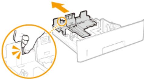
**3 Load the paper so that the edge of the paper stack is aligned against the paper guide on the rear side of the paper drawer.**
