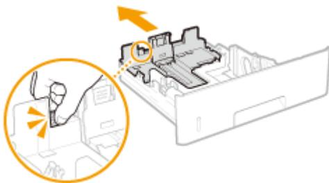
**3 Load the paper so that the edge of the paper stack is aligned against the front side of the paper drawer.**
