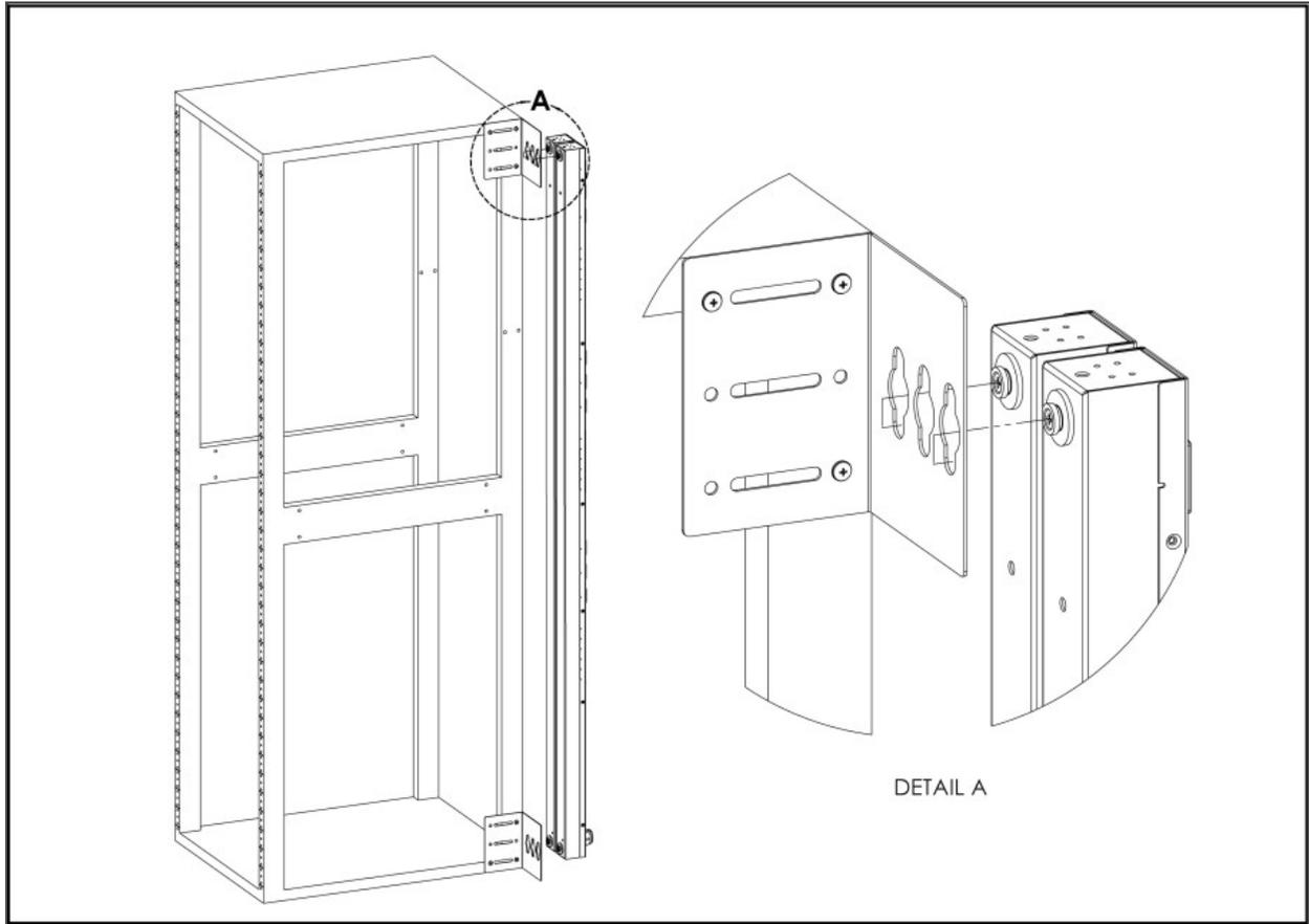
Figure 2.7 Offset/Side-Mount Brackets
