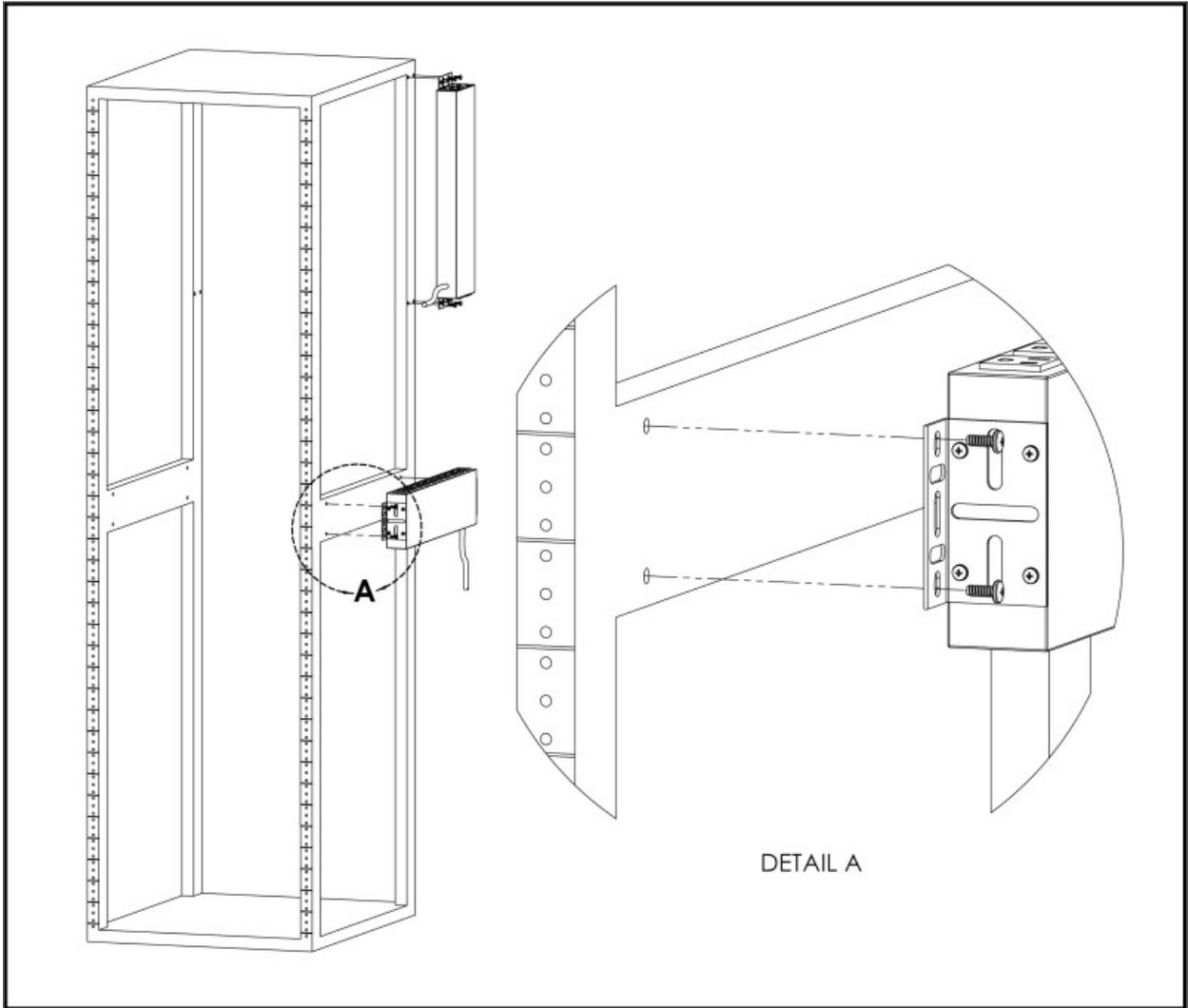
Figure 2.12 23" (inch) Conversion-Mount Brackets
