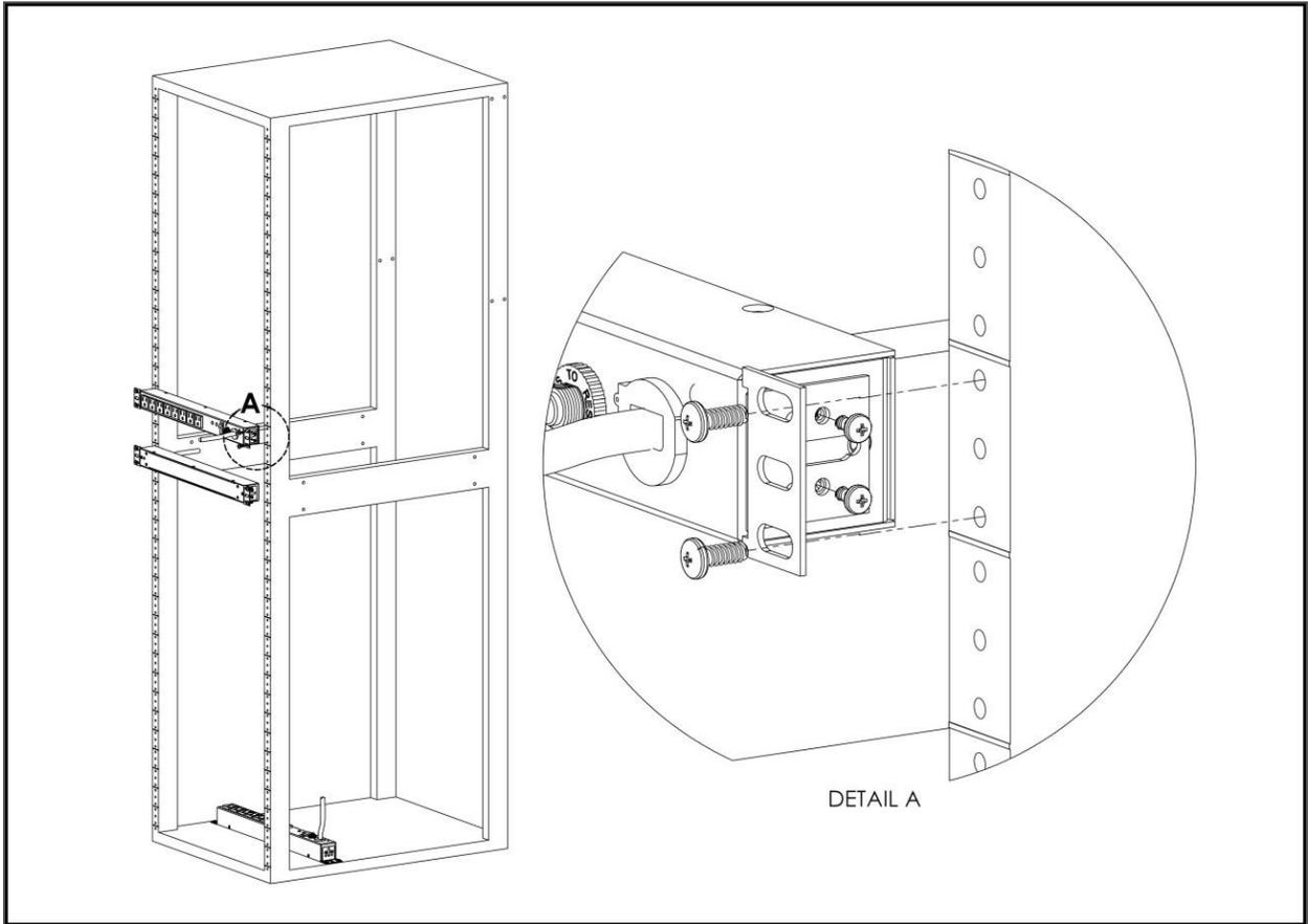
Figure 2.14 Mount Brackets for UPDU with Pivoting End
