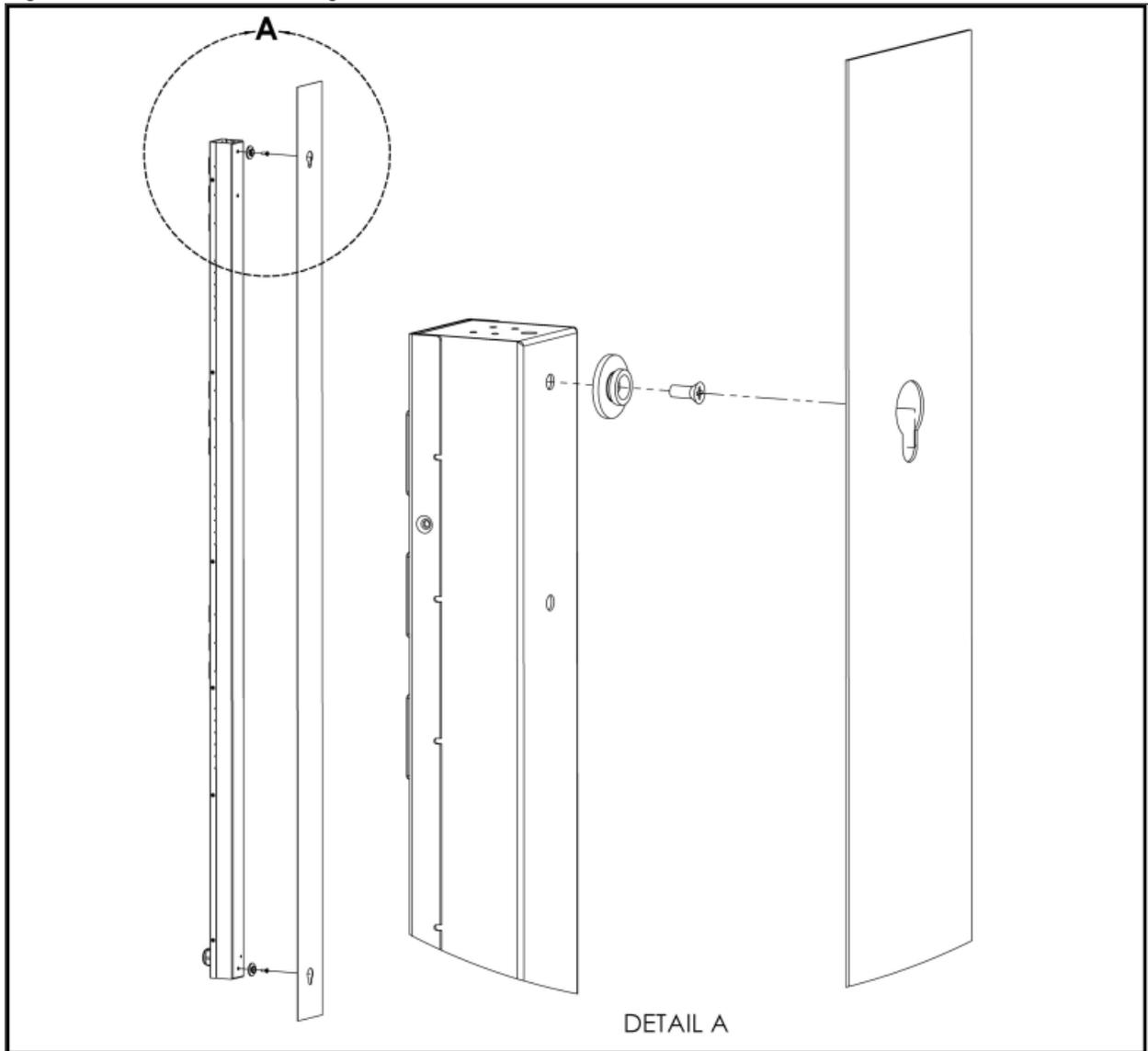
Figure 2.5 Toolless Full-Length Brackets
