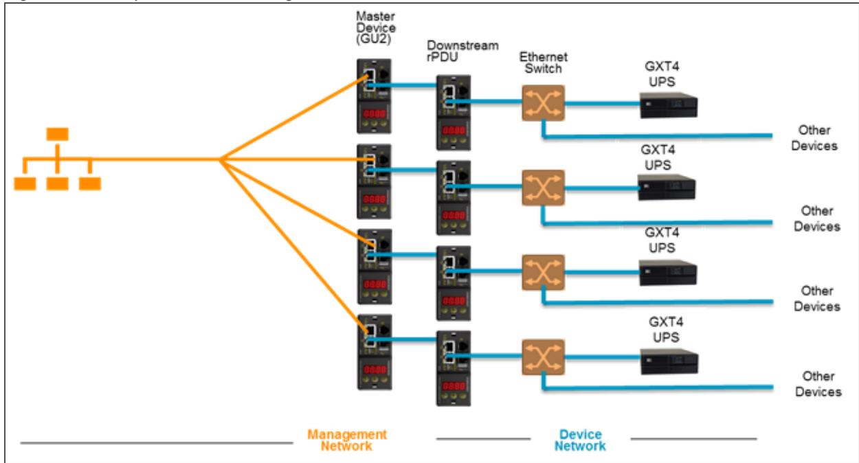
NOTE: RSTP is disabled by default in Geist™ GU1 rPDUs running 3.4.0 or later and Geist™ GU2 rPDUs running 5.3.3 or later. In previous firmware, RSTP is enabled on both platforms. Aggregation does not support RSTP. Leaving RSTP enabled limits an rPDU daisy-chain within aggregation to 40 devices. Disabling RSTP on array devices will remove the 40-device limitation.
