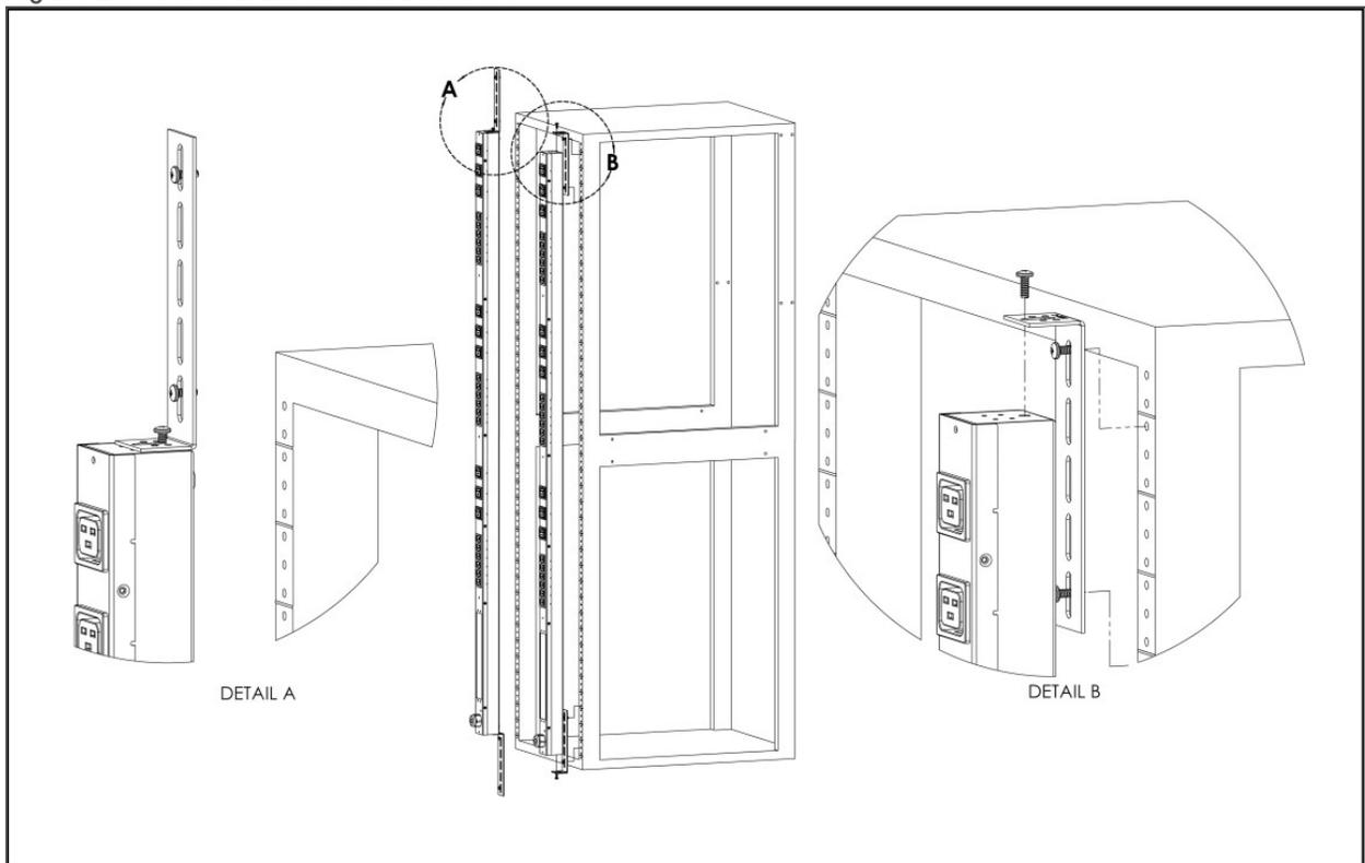
Figure 2.4 Toolless Mounting Hardware
