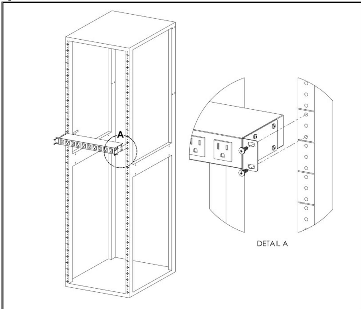
Figure 2.10 Adjustable-Mount Bracket
