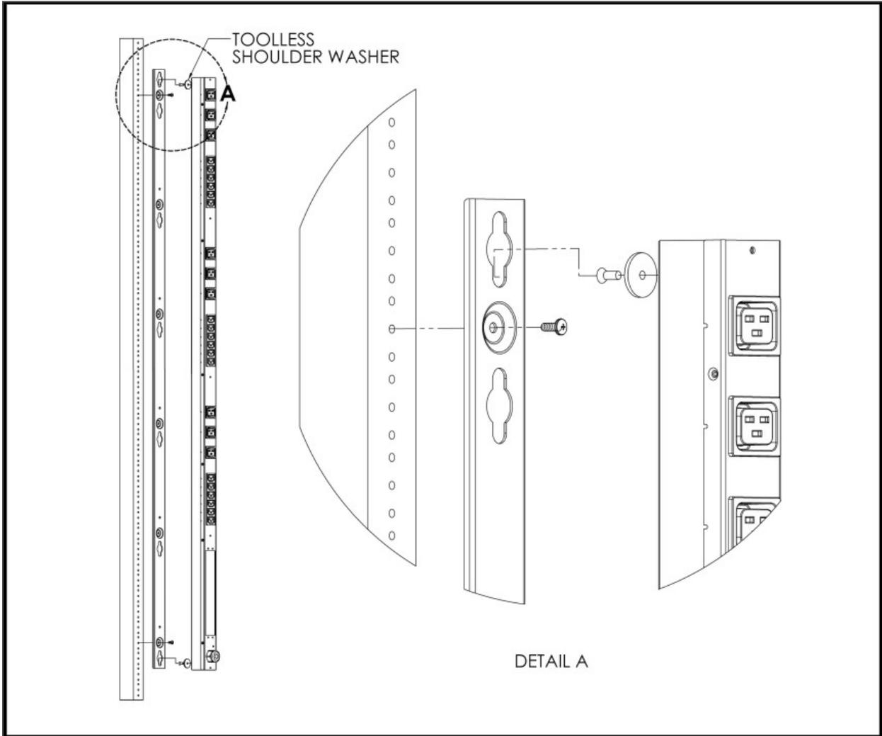
Figure 2.6 Single Side-Mount Two-Units Brackets
