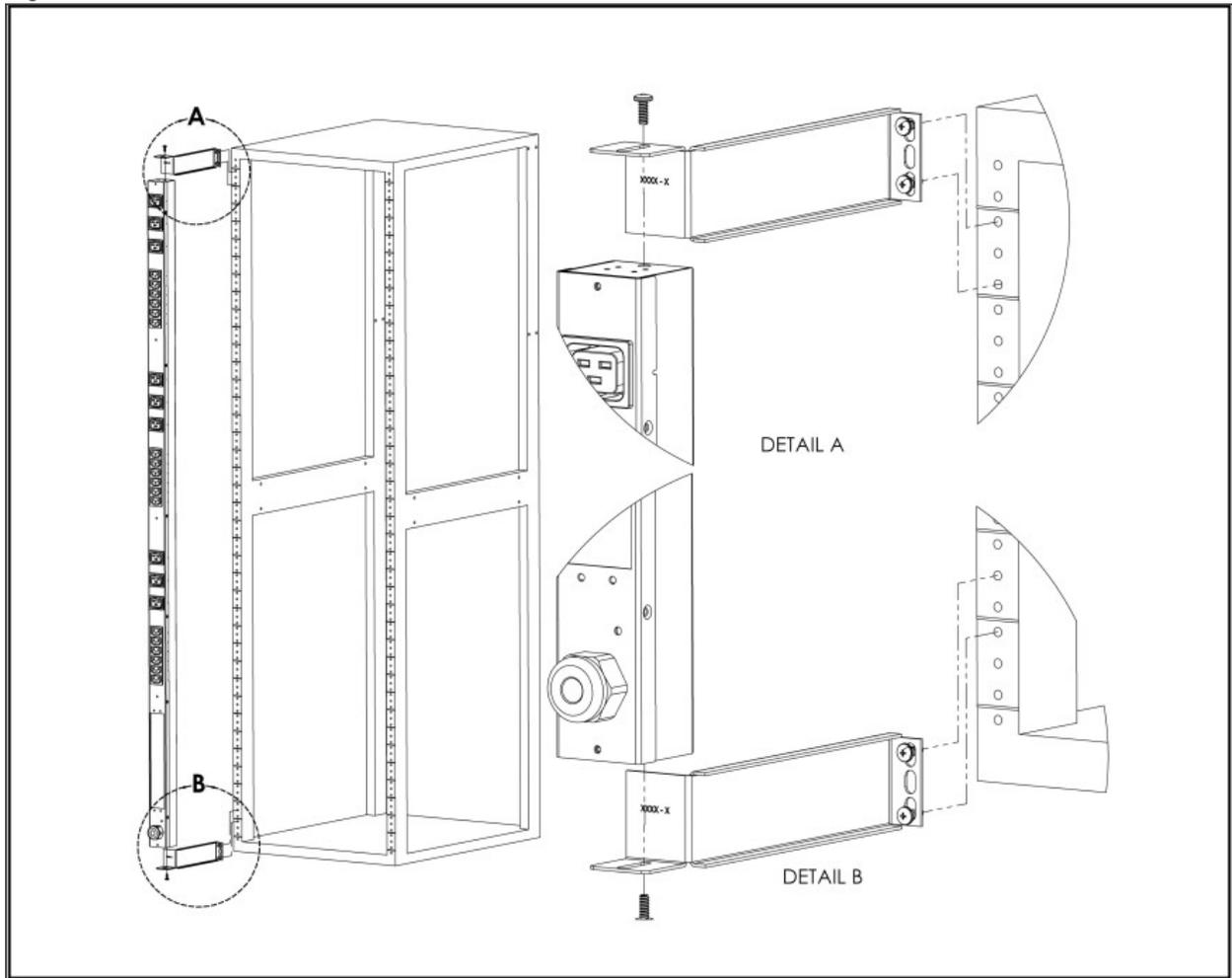
Figure 2.9 Flush-Mount Bracket
