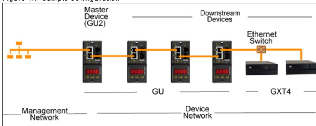
The IMD-3E is the default intelligence card for Vertiv™ Geist™ GU2 rPDUs, which include switched (model numbers beginning with MNS), outlet monitored (model numbers beginning with MNR) and switched plus outlet monitored (model numbers beginning with MNU) products. To serve as the array manager, rPDUs with a legacy intelligence card must first be upgraded to the IMD-3E.
