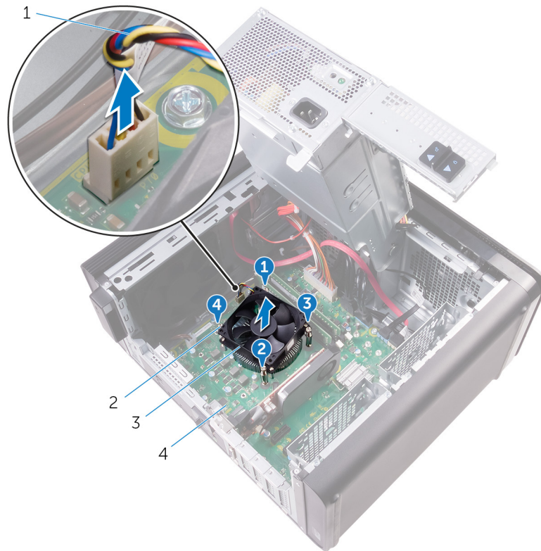
Figure 33. Removing the processor fan and heat sink
