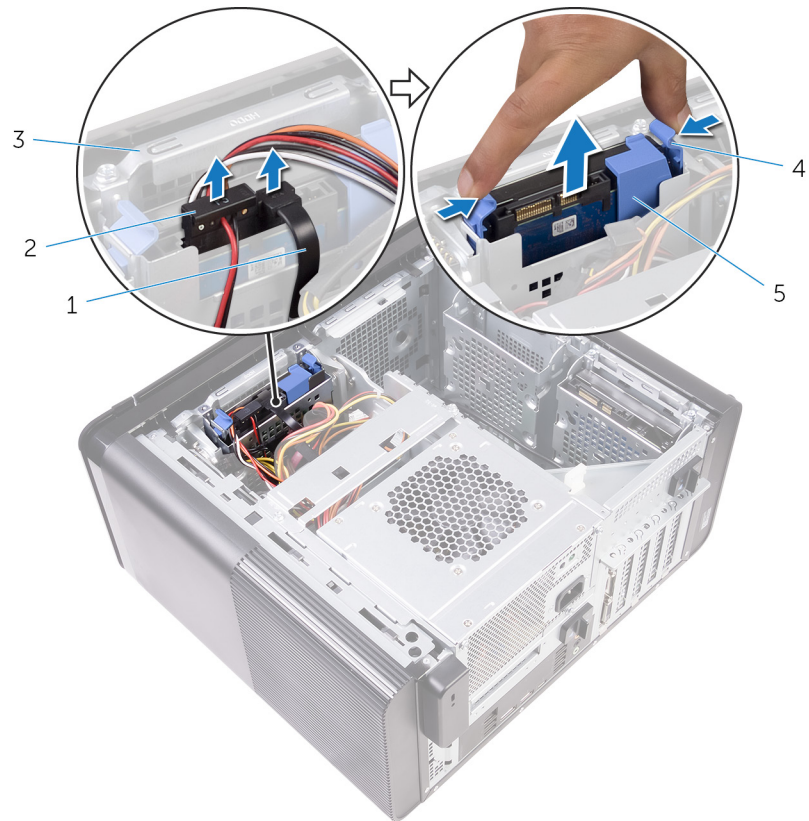
Figure 13. Removing the hard-drive assembly
