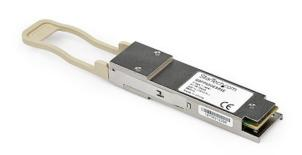
The 3013936-E2-ST is a Citrix 3013936-E2 compatible fiber transceiver module that has been designed, programmed and tested to work with Citrix brand switches and routers. It delivers dependable 40 GbE connectivity over fiber cable, for 40GBASE-SR4 compliant networks, with a maximum distance of up to 100 m (328 ft).
