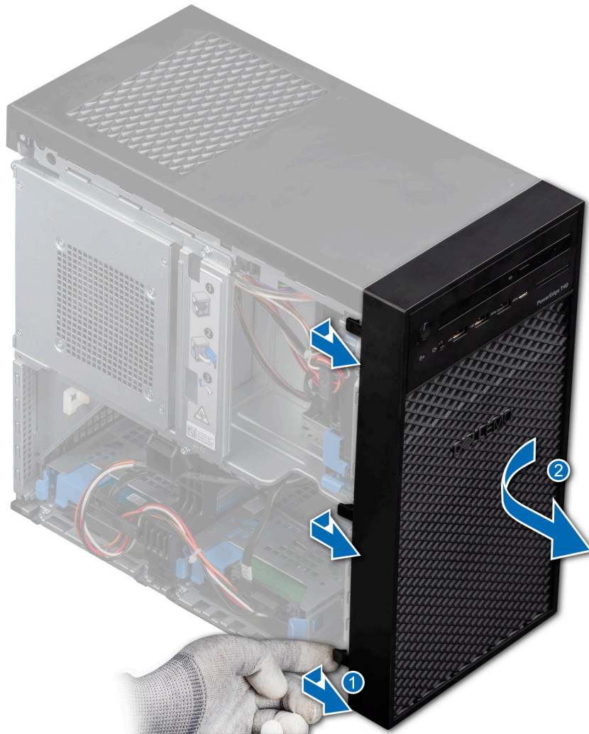
Figure 12. Removing the front bezel
