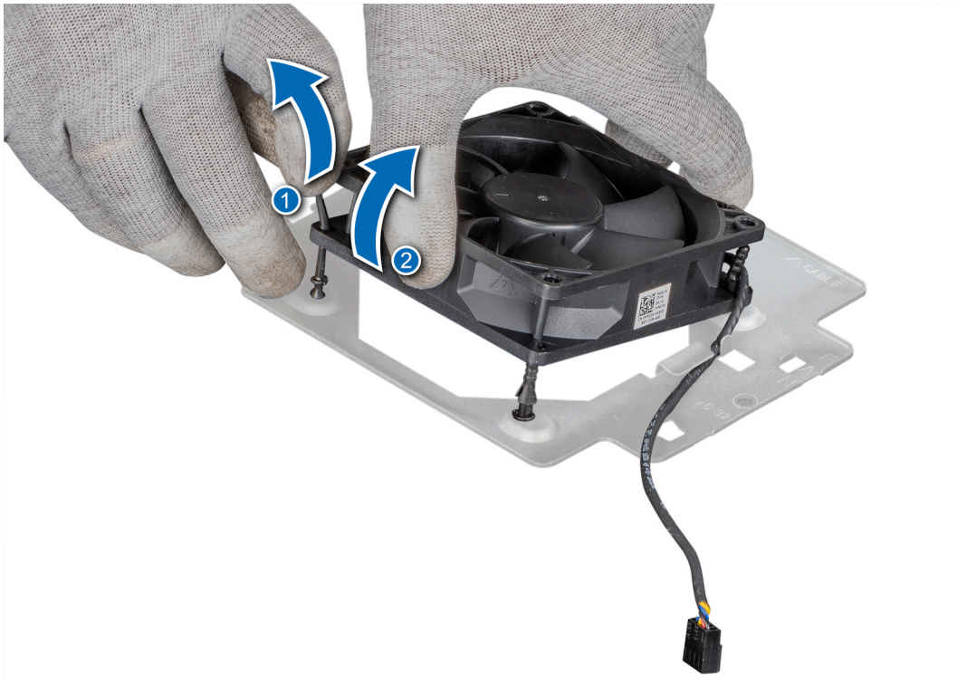
Figure 38. Removing the System fan
