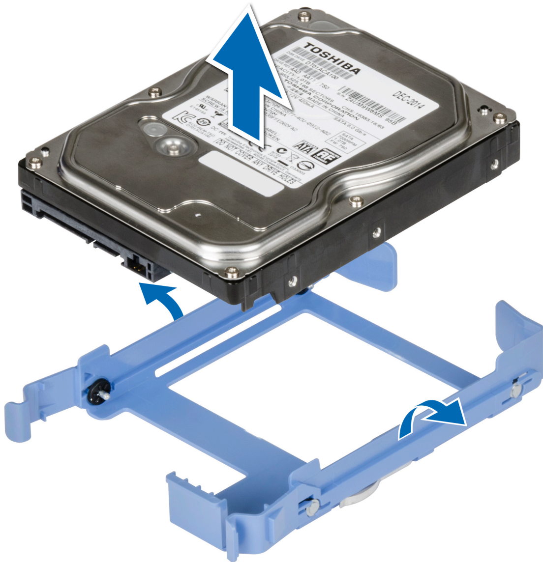
Figure 16. Removing the drive from the drive carrier
