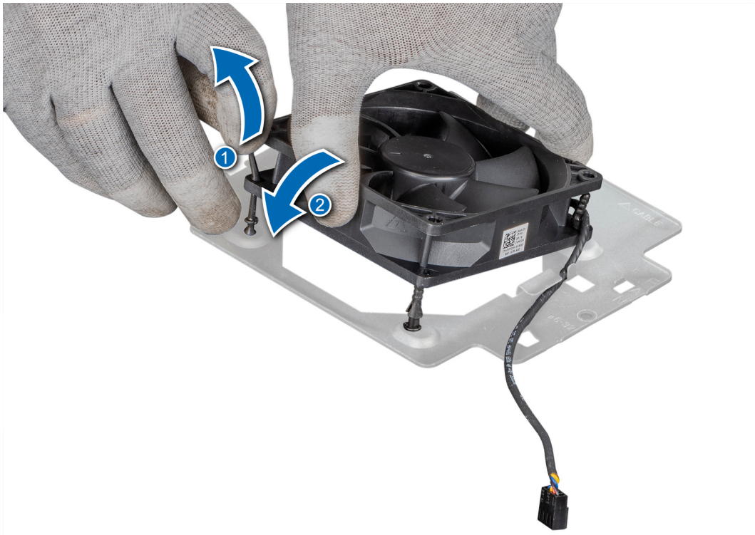
Figure 39. Installing system fan
