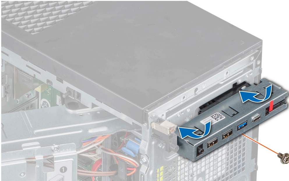
Figure 53. Installing the control panel
