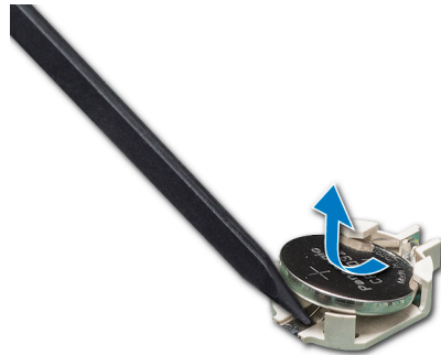
Figure 29. Removing the system battery
