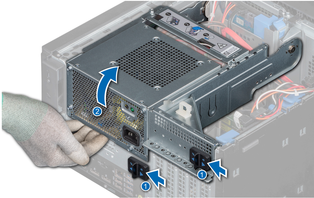
Figure 18. Opening the PSU assembly
