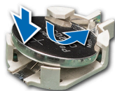
Figure 30. Installing the system battery
