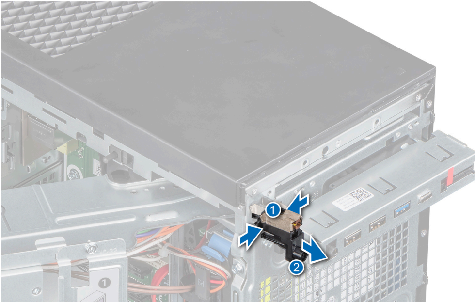
Figure 54. Removing the power button module
