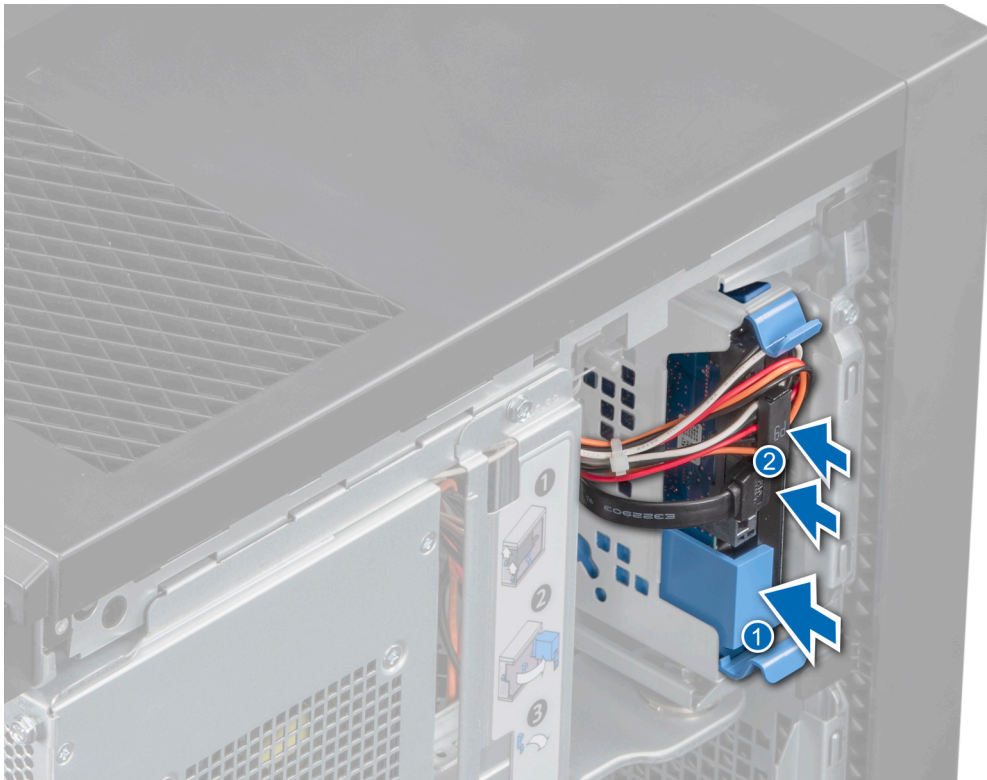
Figure 15. Installing the hard drive carrier
