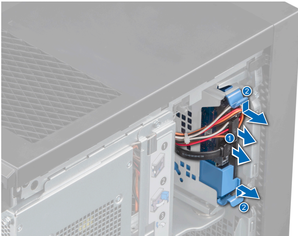
Figure 14. Removing the hard drive carrier
