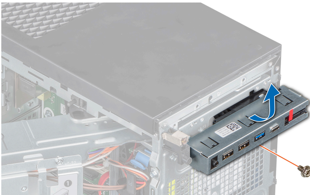
Figure 52. Removal of the control panel
