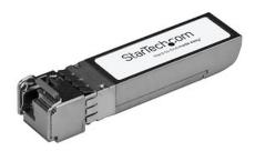
The SFP-10G-BX-U-40-ST is a Cisco SFP-10G-BX-U-40 compatible upstream fiber SFP+ transceiver which pairs with StarTech.com's SFP-10G-BX-D-40-ST. They are designed, programmed and tested to work with 10GBASE-BX compatible Cisco switches and routers. The SFP+ transceiver module supports a maximum distance of up to 40 km (24.8 mi) and delivers dependable 10 GbE connectivity over fiber cabling.
