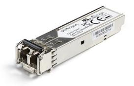
The SFP1FEFXST is a Juniper SFP-1G-ZC compatible fiber transceiver module that has been designed, programmed and tested to work with Juniper brand switches and routers. It delivers dependable 100 Mbps connectivity over fiber cable, for 100BASE-FX compliant networks, with a maximum distance of up to 80 km (49.7 mi).
