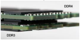
Figure 2. Thickness difference
