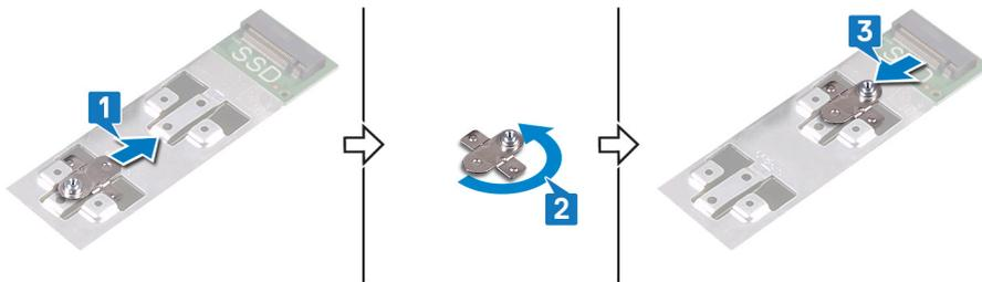
4. Align the notch on the solid-state drive/Intel Optane memory module with the tab on the solid-state drive slot.
