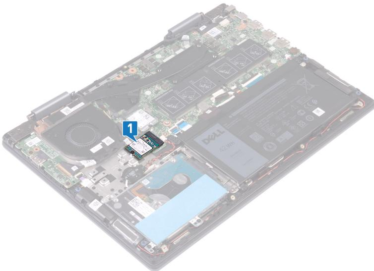
2. Remove the screw (M2x3) that secures the solid-state drive/Intel Optane memory module to the palm-rest and keyboard assembly.
