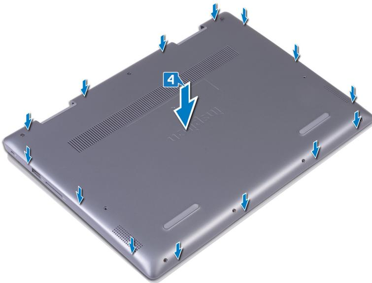
5. Tighten the three captive screws that secure the base cover to the palm-rest and keyboard assembly.
