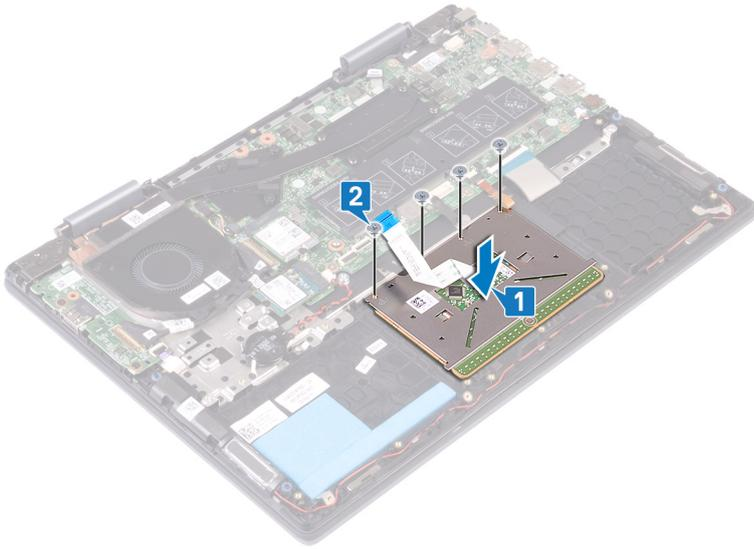
3. Align the screw holes on the touchpad bracket with the screw holes on the touchpad.
