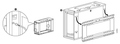
3. **NOTE:** Skip this step for concrete or cinder block. Use a stud finder to locate and mark at least two (2) wall studs. Hold the bracket to the wall so that four (4) fastener holes are aligned with the studs. Ensure the bracket is horizontally level and install two (2) drywall screws as shown.
