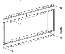
**NOTE:** The drywall screws will hold the bracket in position while you secure the bracket so that it can bear the weight of the cabinet. Do not put any weight on the bracket at this time.
