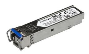
The SFPGE40KT3R5 is a Juniper SFPP-10GE-SR compatible fiber transceiver module that has been designed, programmed and tested to work with Juniper brand switches and routers. It delivers dependable 1 GbE connectivity over fiber cable, for 1000Base-BX40-U compliant networks, with a maximum distance of up to 40 km (24.8 mi).
