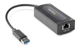
Add 5G network access to your laptop, using a USB A port. This USB 3.0 Type A to Gigabit network adapter gives you wired Ethernet network and Internet access. The NBASE-T adapter is 4-speed compatible, including IEEE 802.3bz (2.5G/5GBASE-T), IEEE 802.3U (100BASE-TX) and 802.3ab (1000BASE-T).
