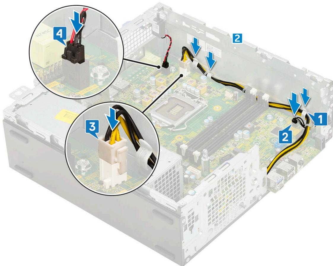
6. Connect the power cable, optical drive data cable and hard drive data cable [1, 2, 3].
