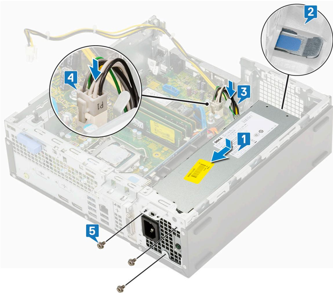
5. Route the CPU power cable through the retention clips [1].
