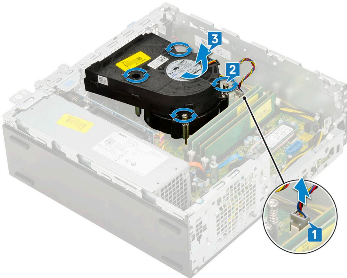
**NOTE:** Loosen the screws in a sequential order (1,2,3,4) as mentioned on the system board.
