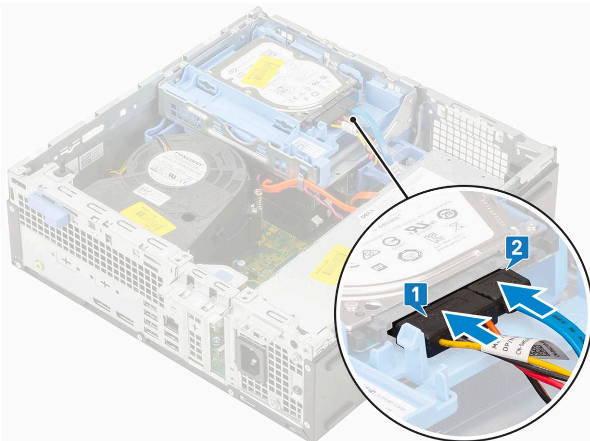
5. Slide the release tab to lock the module [2].
