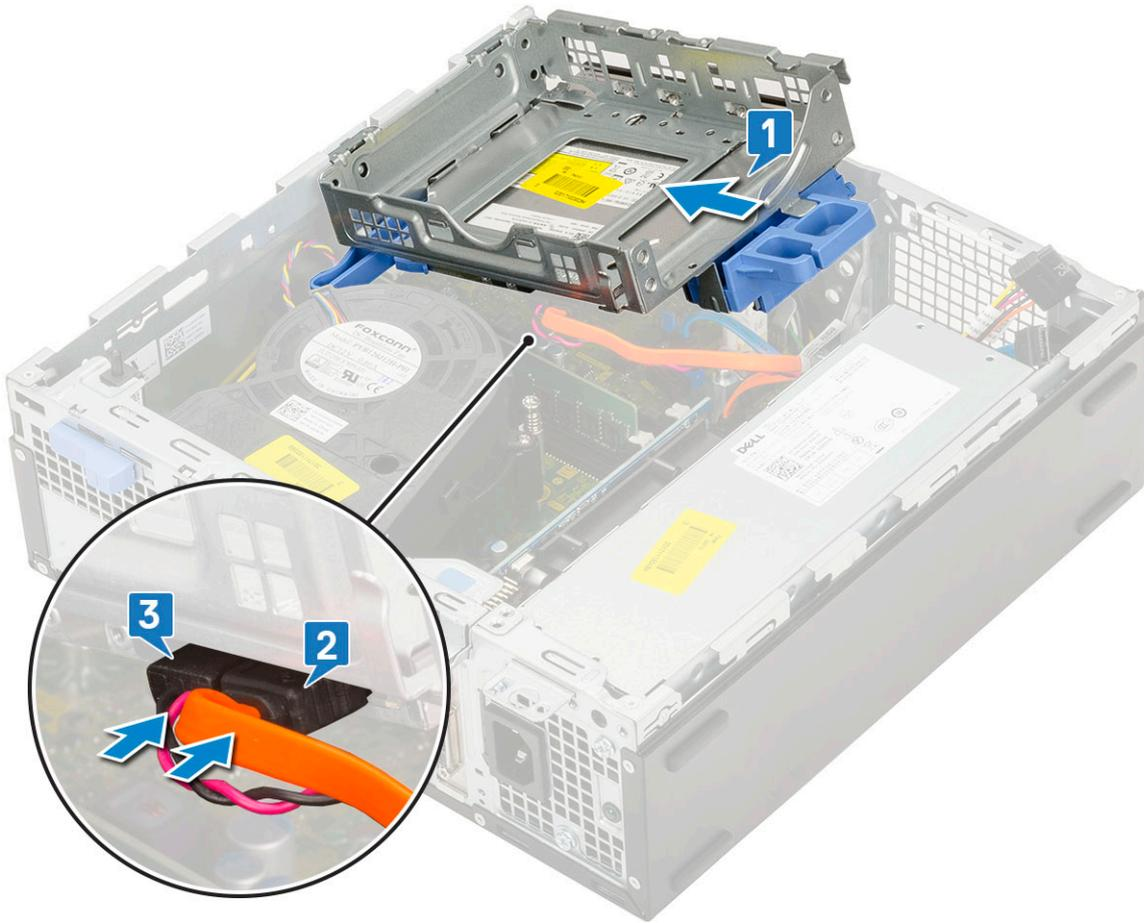
3. Lower the hard drive and optical drive module so that it is placed in its slot [1].
