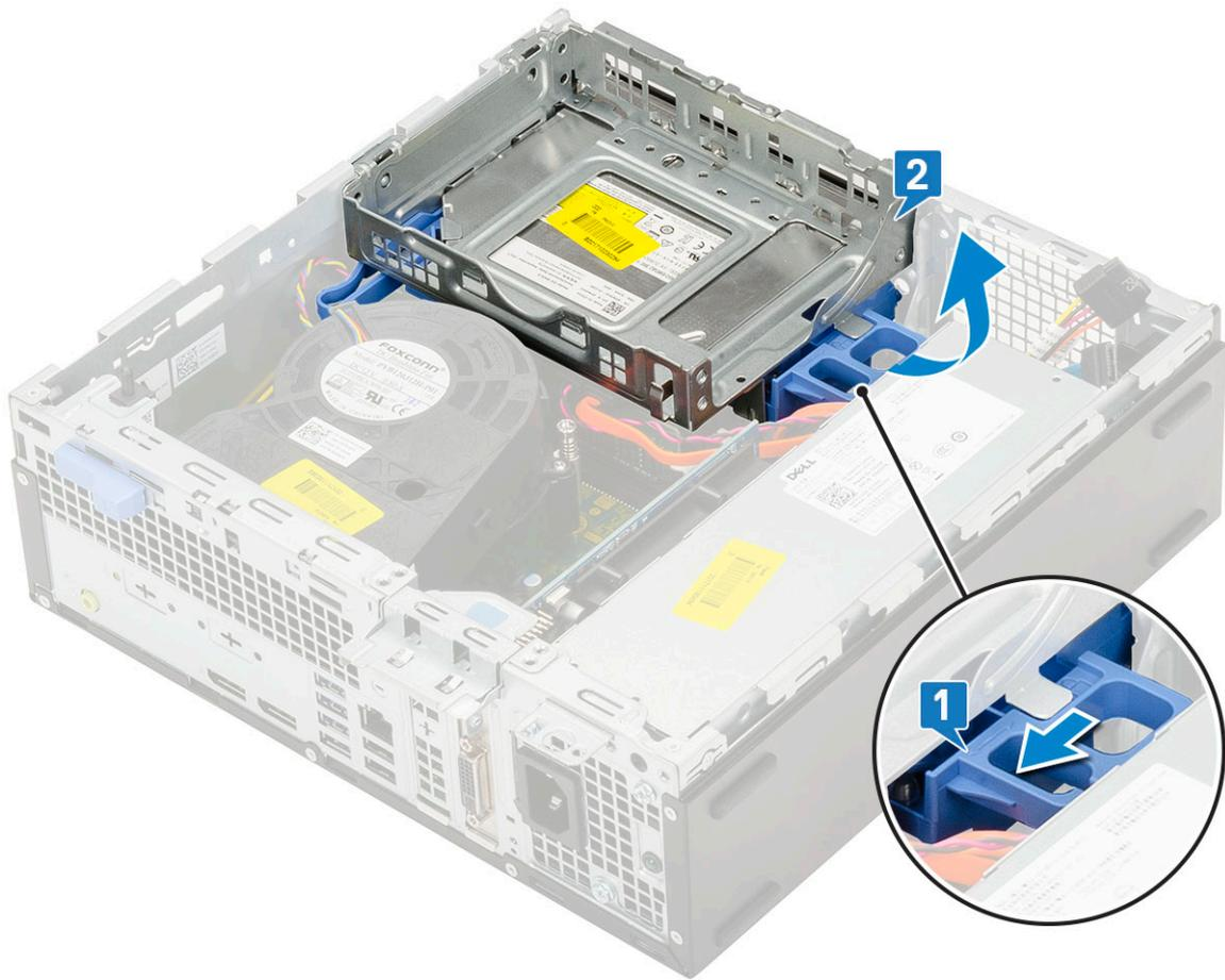
4. To remove the hard drive and optical drive module:
