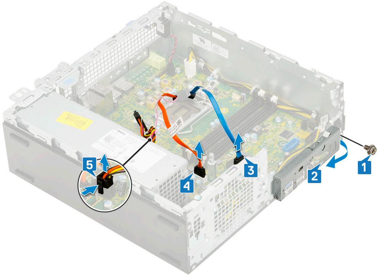
5. Disconnect the following cables from the connectors on the system board:
