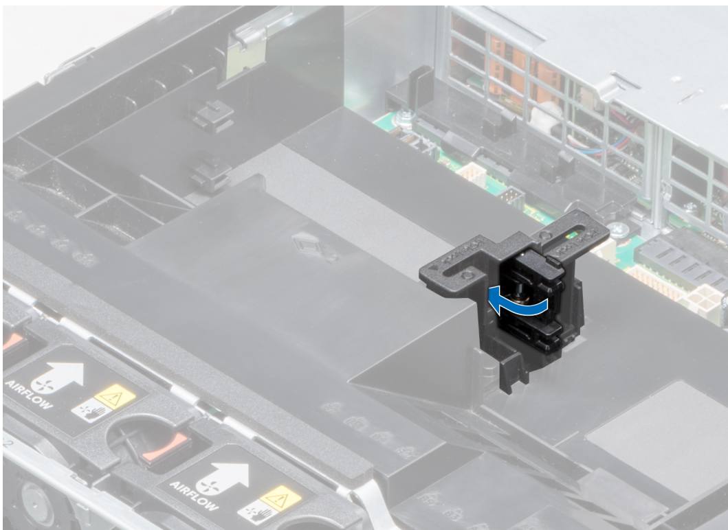
Figure 66. Closing the PCIe card holder latch
