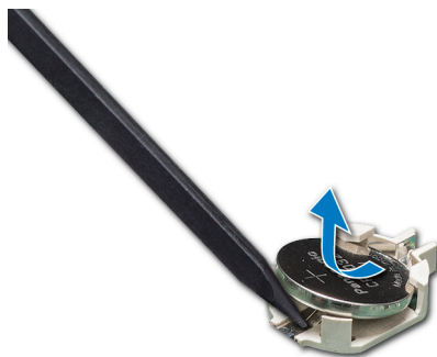
Figure 121. Removing the system battery
