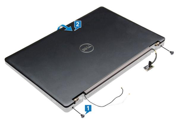
7 Slide upward the display assembly away from the system base.
