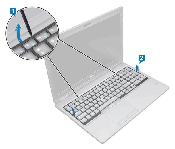
(i) NOTE: Use a plastic scribe to pry the keyboard lattice from the pry points and move around the lattice for removal.
