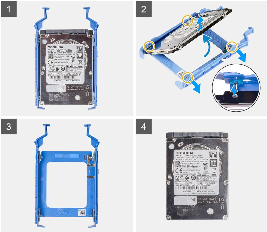
3. Pry the hard-drive carrier to release the tabs on the assembly from the slots on the hard drive.
