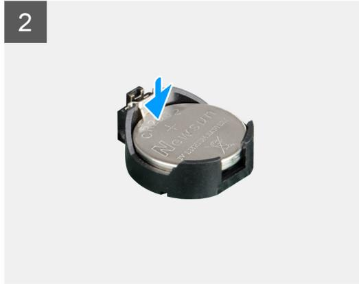
Insert the coin-cell battery into the socket with the positive side (+) labeled facing up and snap the battery in the socket.
