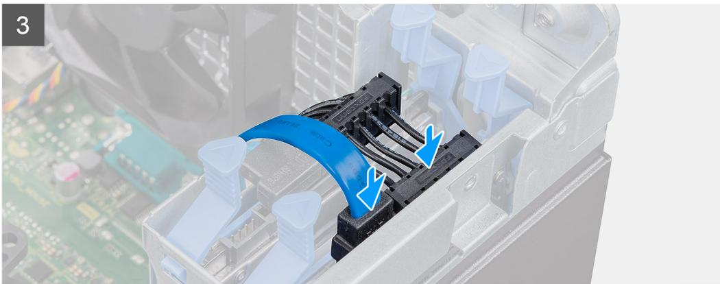
3. Slide the hard-drive assembly into the hard-drive cage until it snaps into place.
