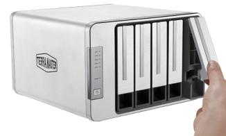
3. After the tray is fully inserted, the handle should be closed. The hard disk installation is completed. If you would like to install the remaining hard disks you have, please refer to steps above.
