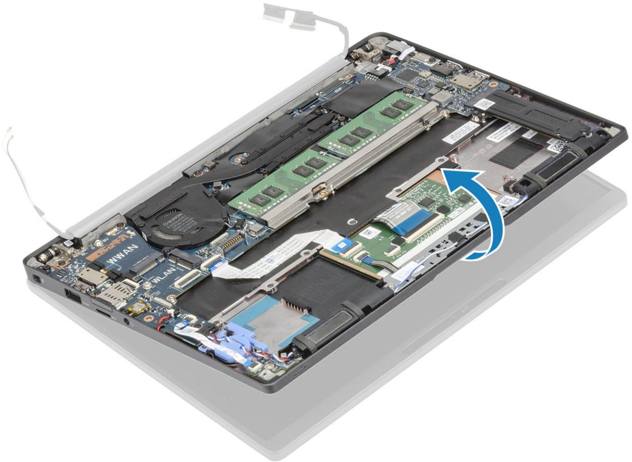
2. Remove the six (M2.5x4) screws [1] and remove the display assembly from the palmrest assembly [2].
