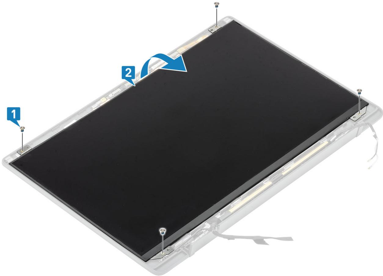
2. ⓘ **NOTE: Do not pull and release the Stretch (SR) tapes from the display panel. There is no need to separate the brackets from the display panel.**
