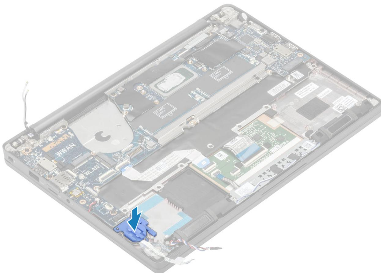
9. Connect the power button (with finger print reader) cable to the system board [1].
