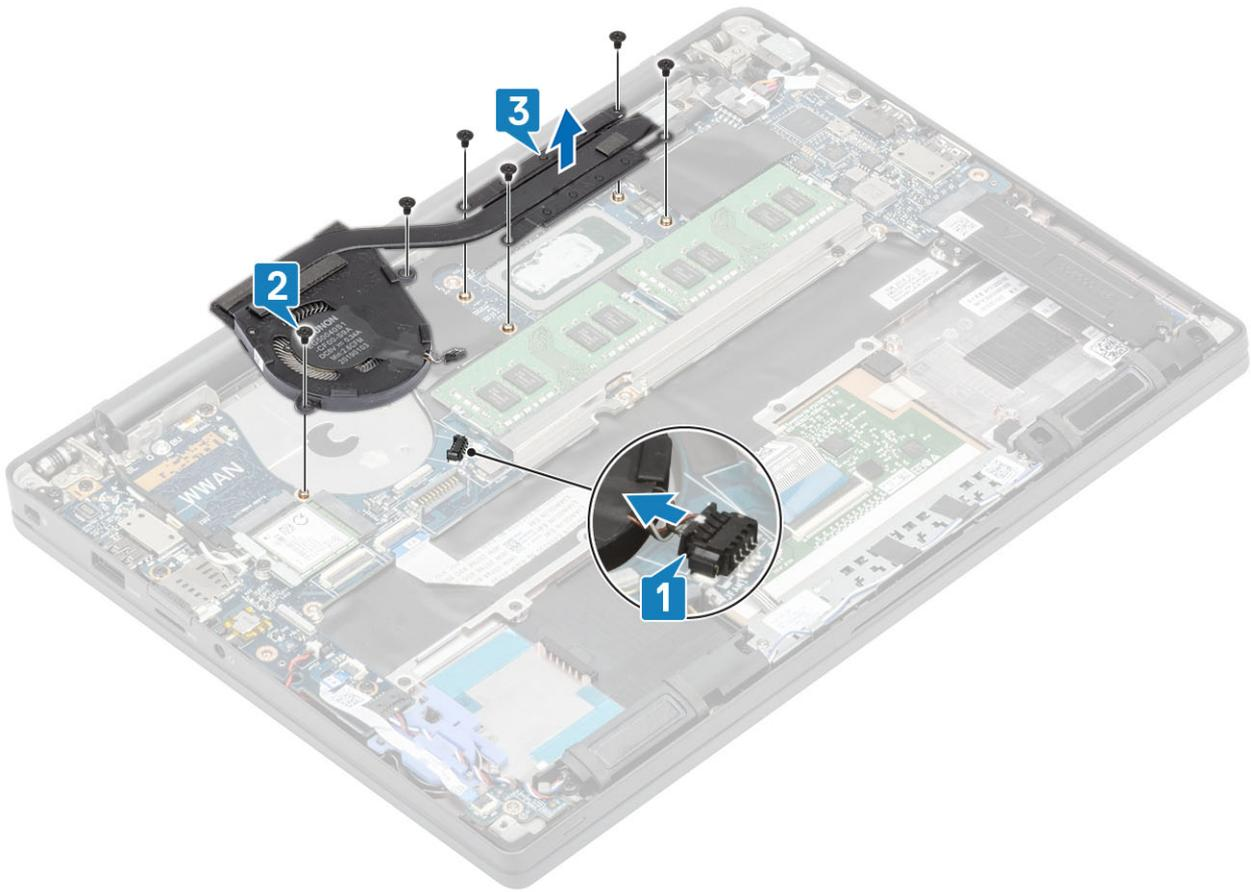
4. Remove the single screw securing the fan to heatsink.
