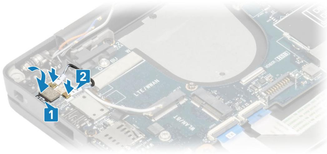
11. Route the speaker cable along the tab [1] beside the LED daughterboard and connect it to the system board [2].
