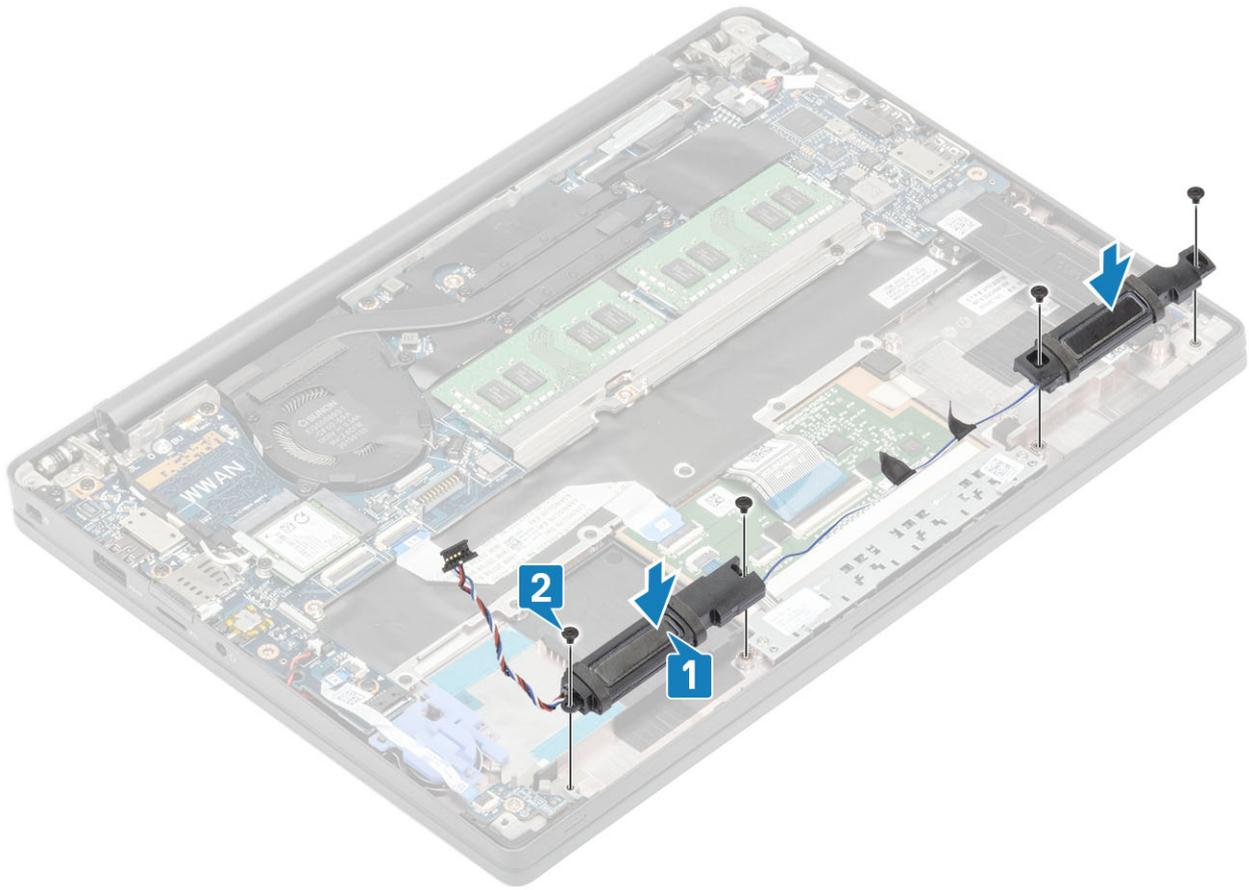
3. Adhere the tape to secure the speaker cable on the touchpad button board [1].
