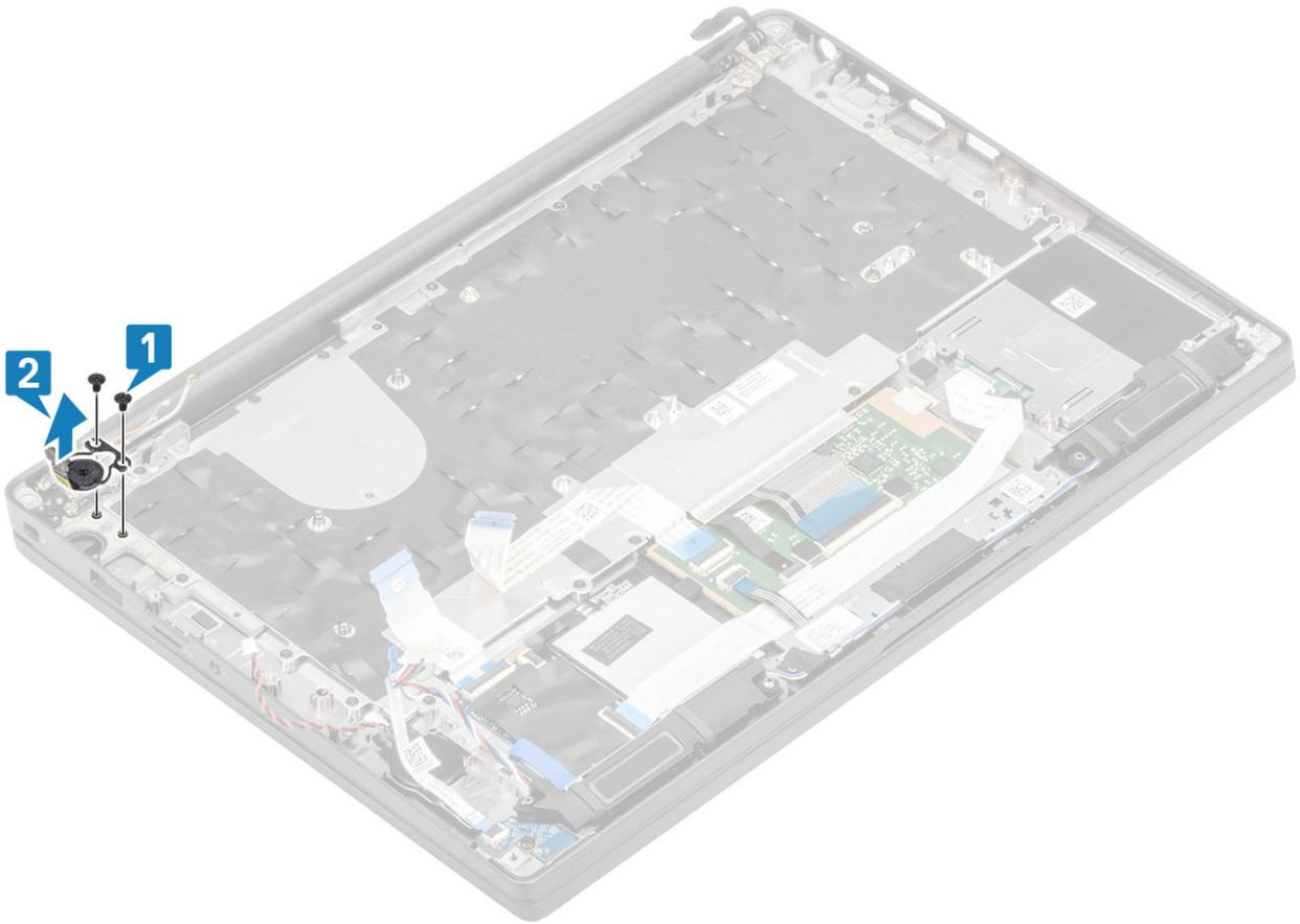
Figure 4. Removing the power-button board with FPR
