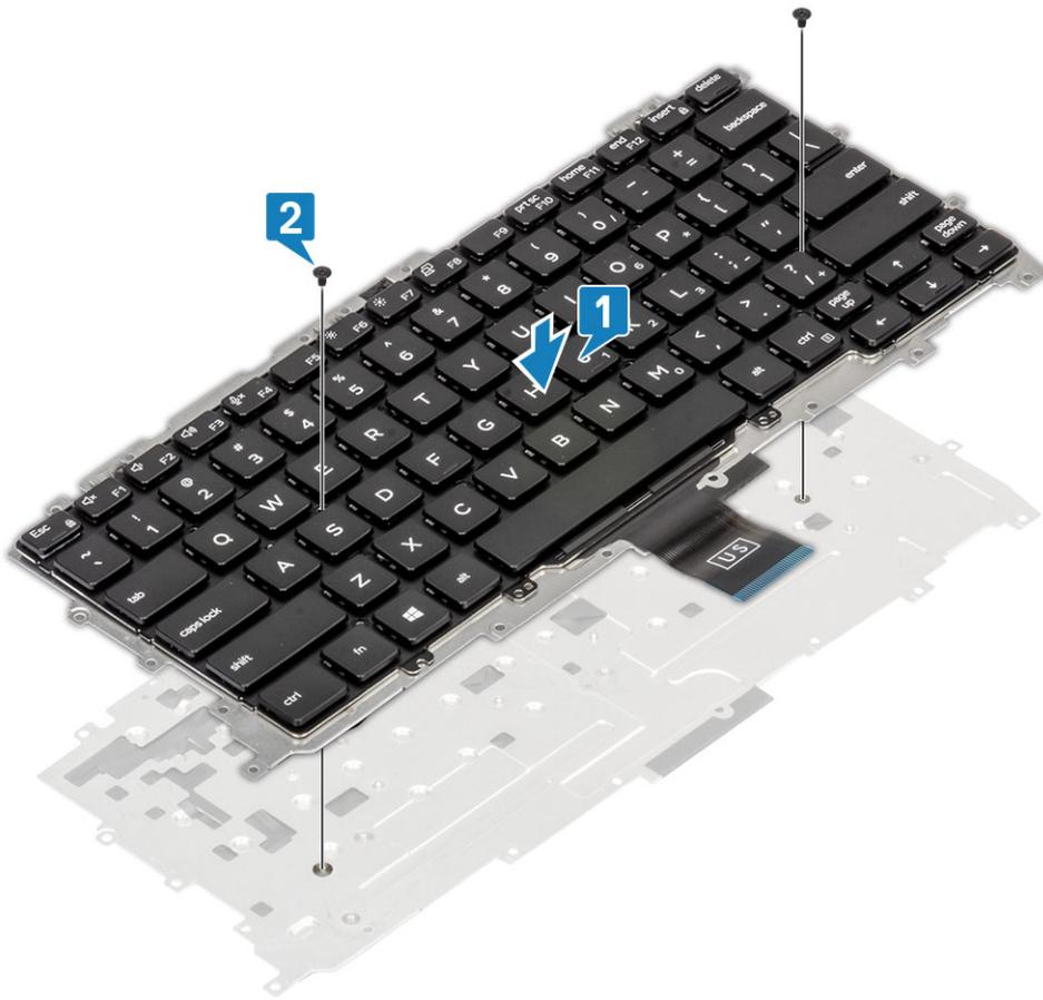
2. Place the keyboard assembly in the palmrest [1] and secure it with the 19 (M1.6x2) screws [2].
