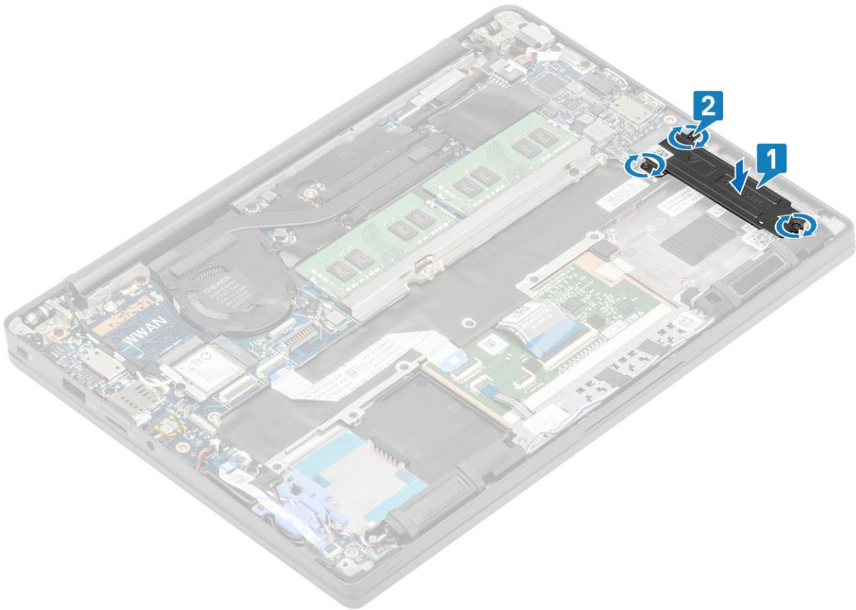
**NOTE:** This procedure illustrates a M.2 2280 SSD. M.2 2230 SSD requires a special bracket and plate to secure it to the palmrest assembly.
