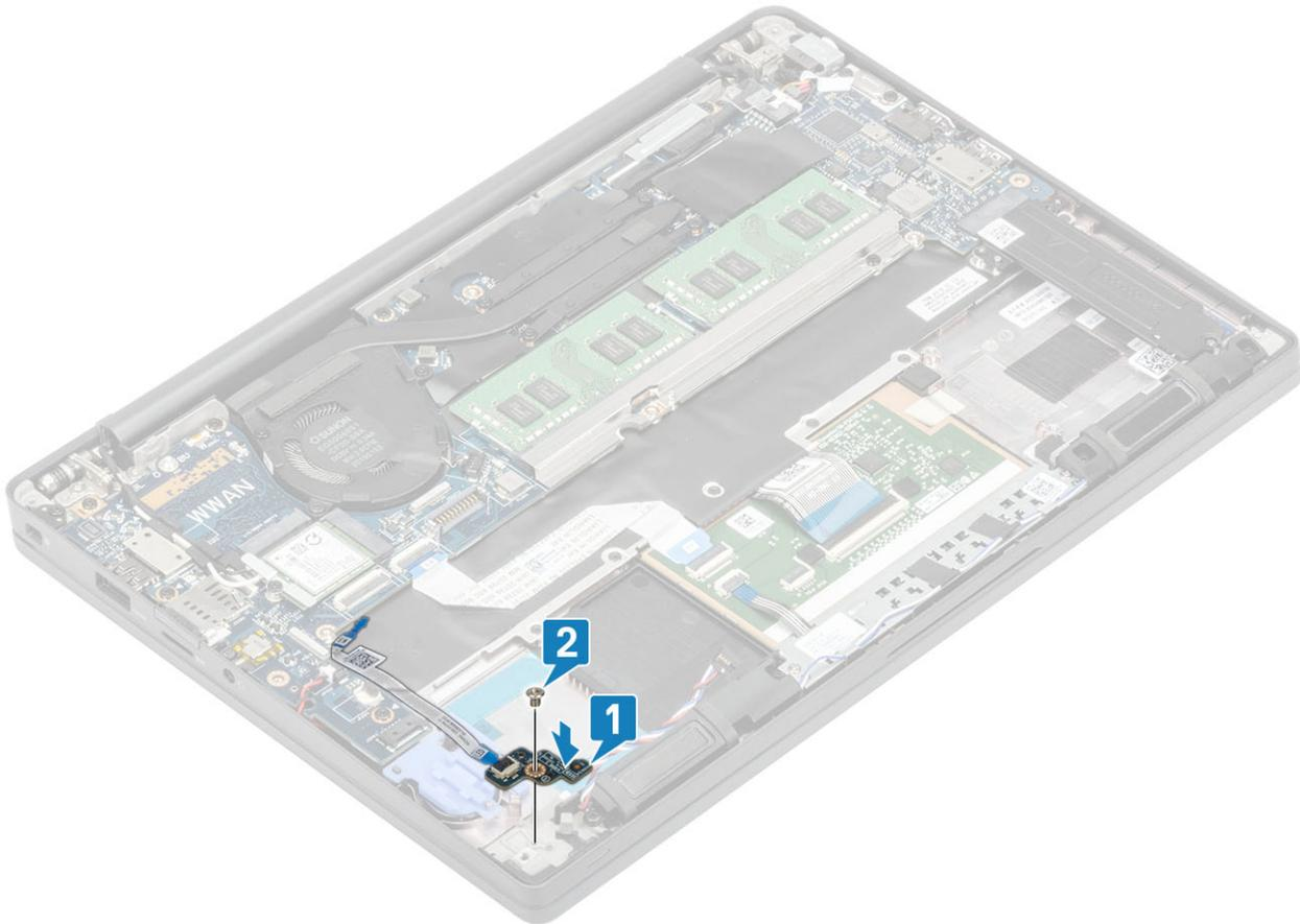
3. Route the LED board ribbon cable over the rubber routing channel on the coin cell [1].
