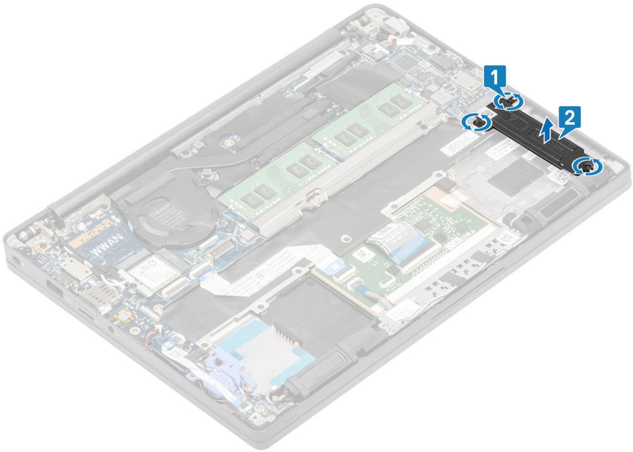
3. Slightly lift and remove the SSD out from its connector on the system board.
