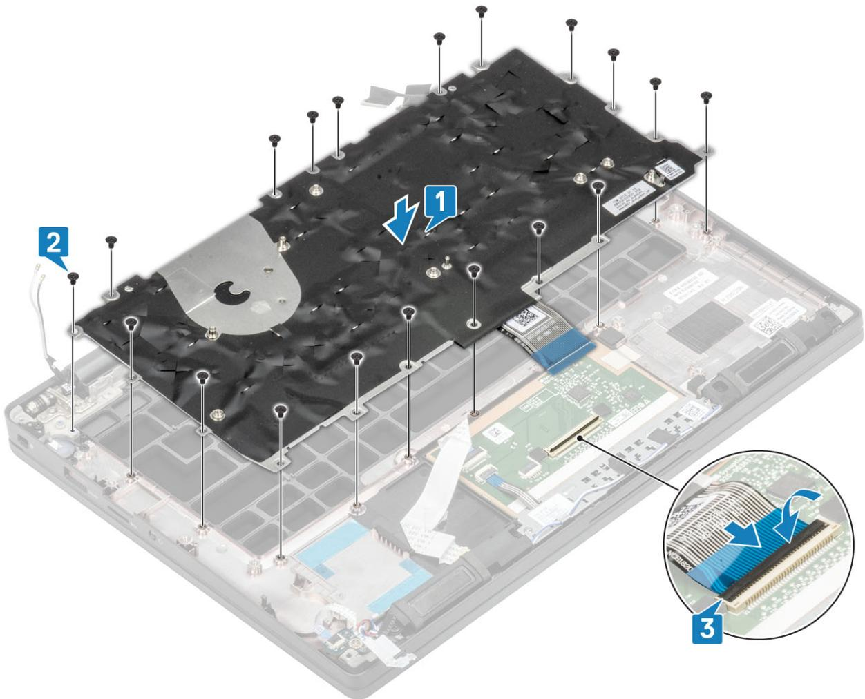
**NOTE:** Backlit keyboards have an extra backlight cable to be connected to the touchpad module.
