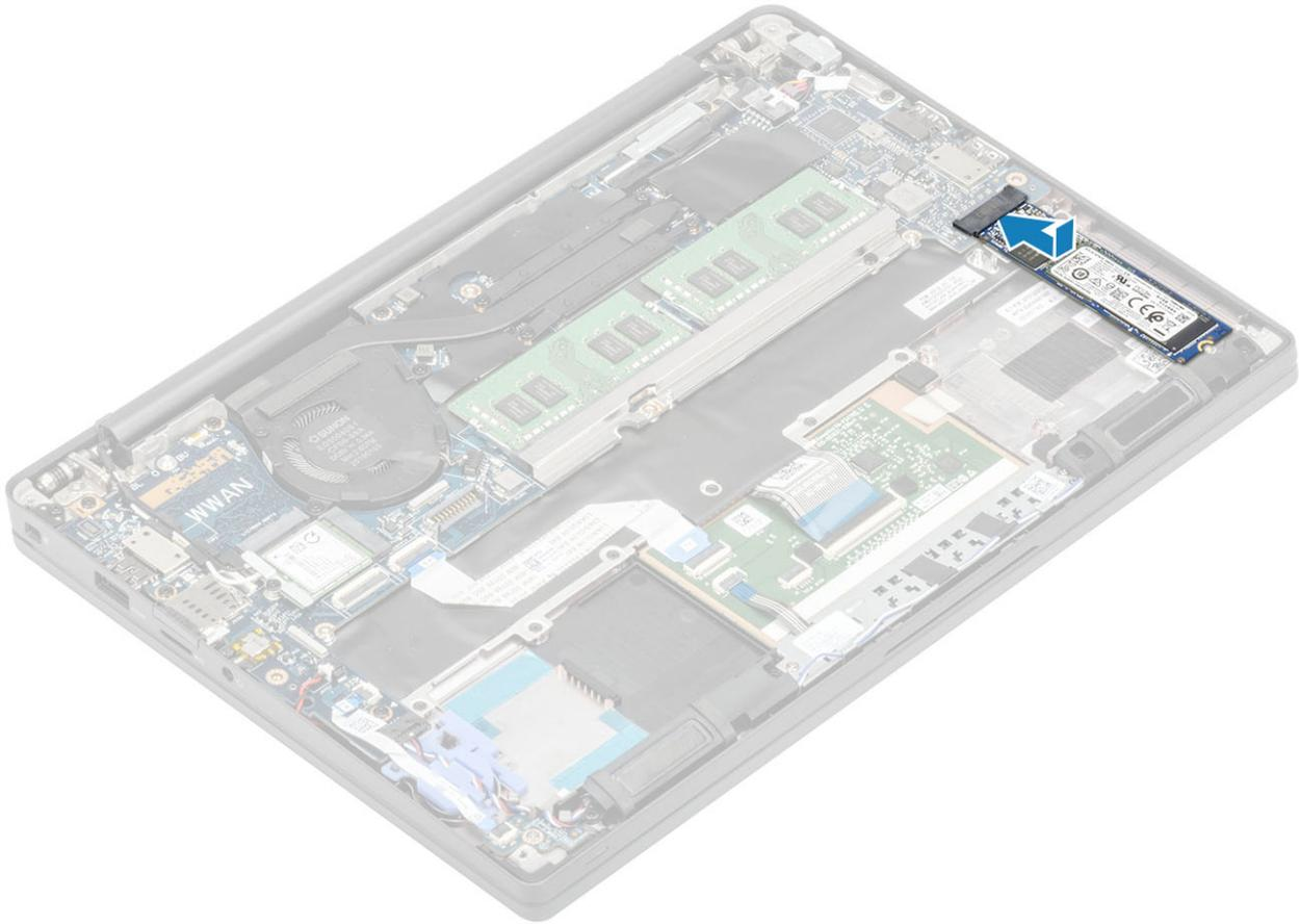
2. Place the SSD plate pre-installed with thermal sticker on the underside over the SSD [1].
