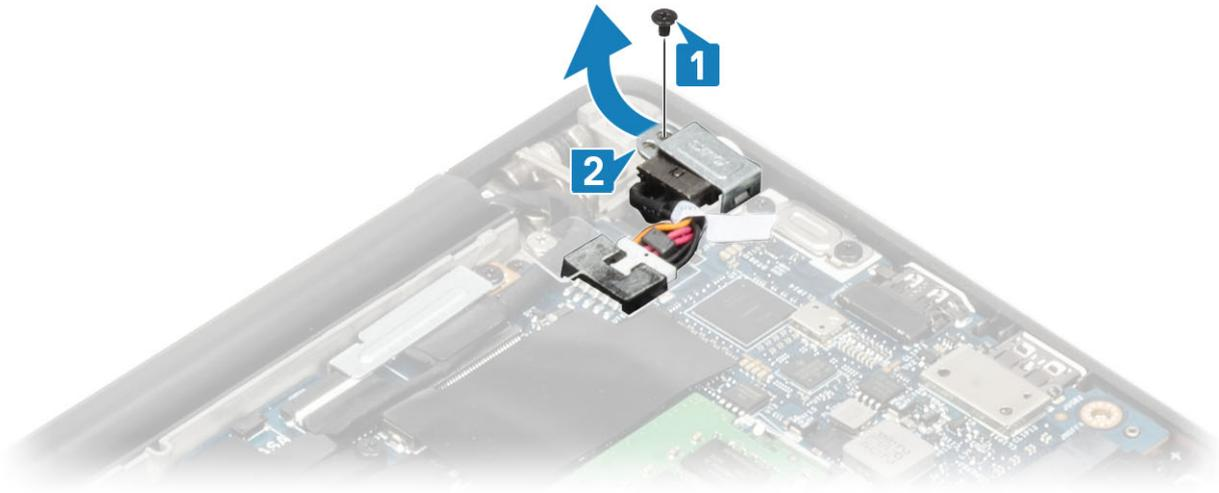
3. Disconnect the power adapter port cable from the system board [1].
