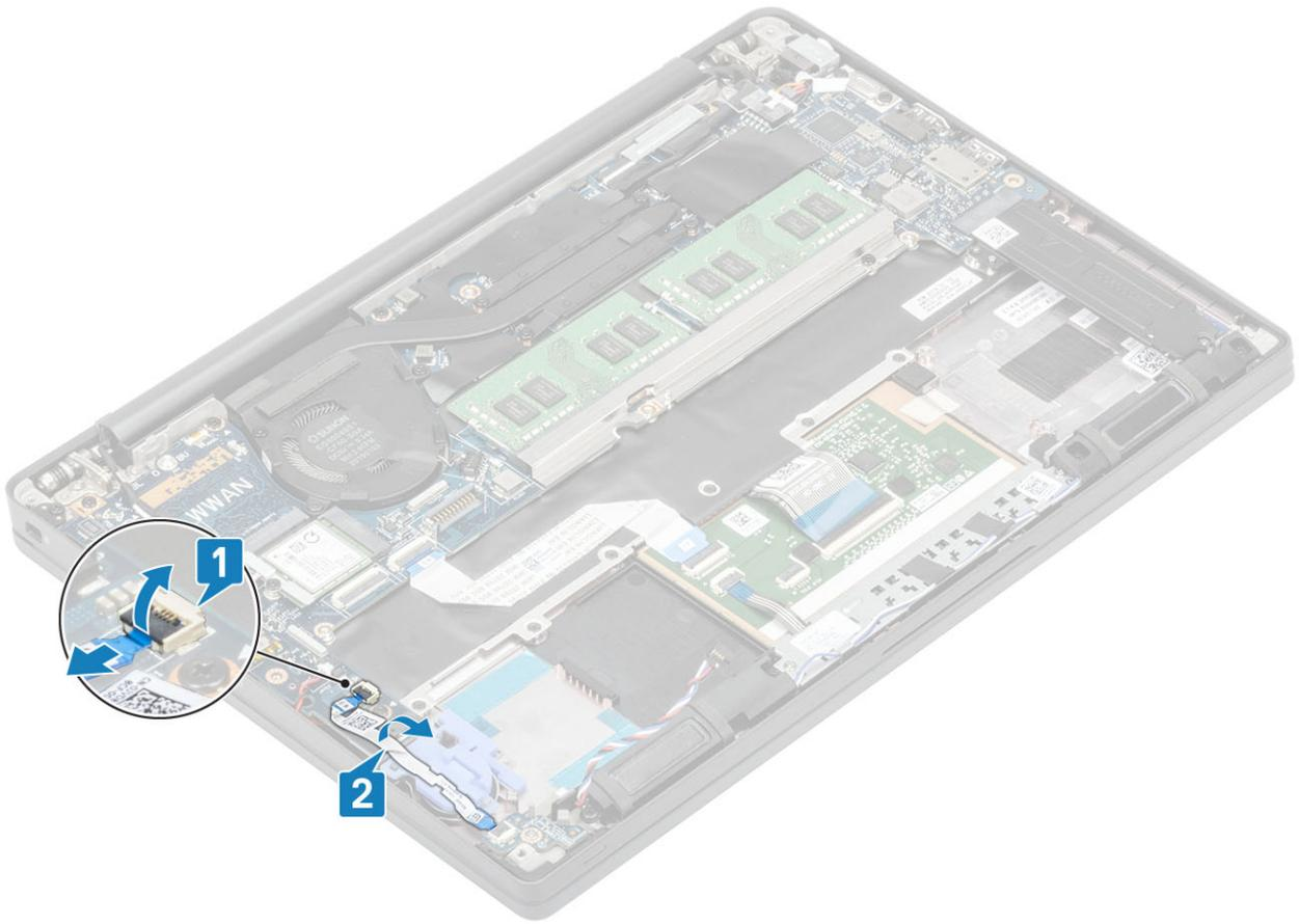
3. Remove the single (M2x2.5) screw [1] and remove the LED daughterboard from the palmrest assembly [2].
