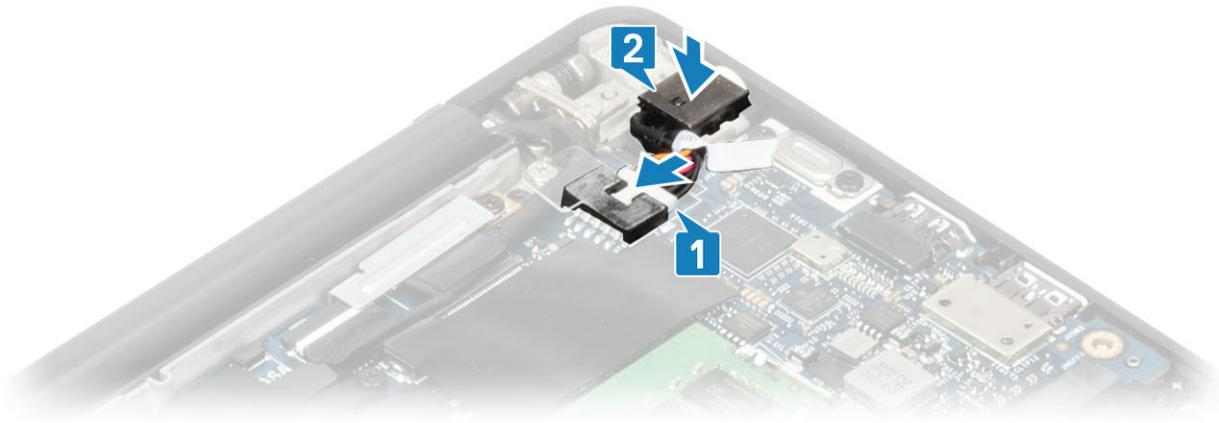
3. Replace the metal bracket over the power adapter port [1].
