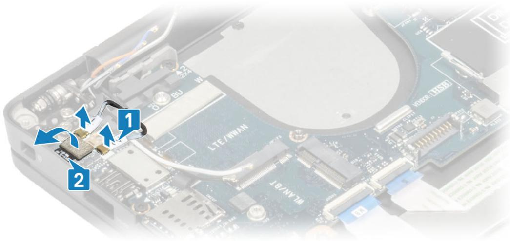
13. Remove the two (M2x4) screws [1] and lift up the USB Type-C bracket from the system board [2].
