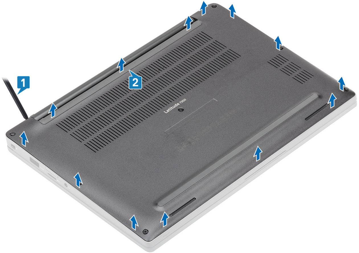
4. Lift and remove the base cover from the computer.
