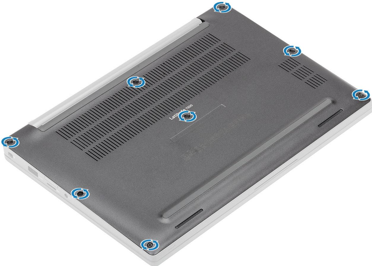
2. Use a plastic scribe to pry the base cover at the indents near the left and right hinges [1].
