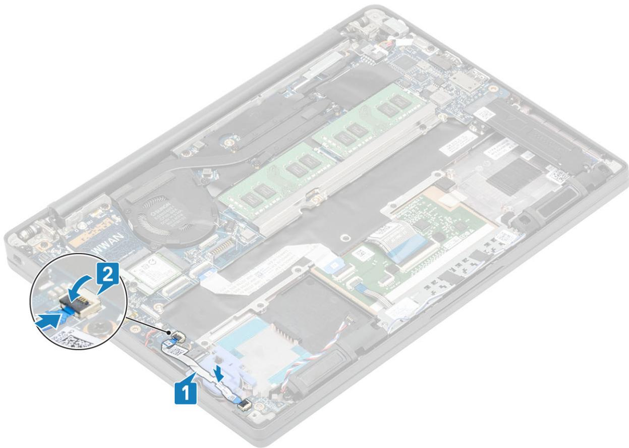
**CAUTION:** Route the speaker cable [1] over the LED daughterboard and then connect it to the system board [2] to prevent damage to the speaker cables.
