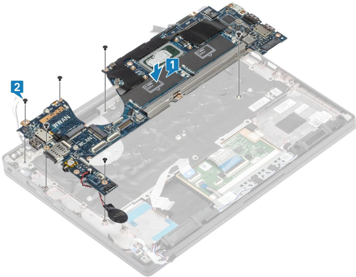
**NOTE:** For models shipped with a fingerprint reader or WWAN antennas, there are four (M2x3) screws securing the system board to the computer.
