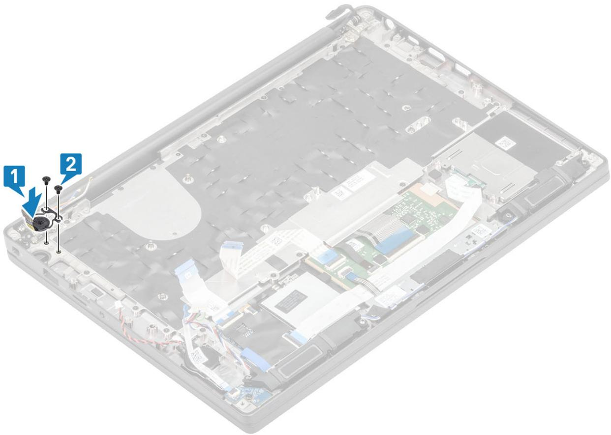
**Figure 6. Installing the power-button board with FPR**
