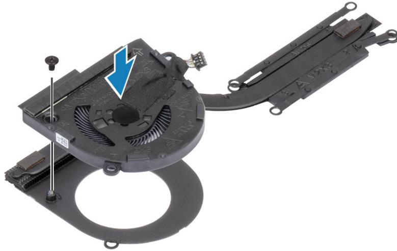
2. Place the heatsink fan assembly in the computer [1].
