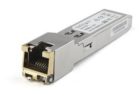
The SFP1GEFEETST is a Juniper SFP-1GE-FE-E-T compatible copper transceiver module that has been designed, programmed and tested to work with Juniper brand switches and routers. It delivers dependable 1 GbE connectivity over copper cable, for 10/100/1000BASE-T compliant networks, with a maximum distance of up to 100 m (328 ft).
