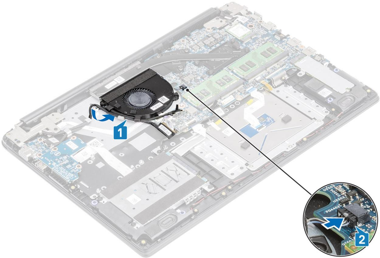
5 Connect the VGA board cable [1], and the display cable to the system board [2].
