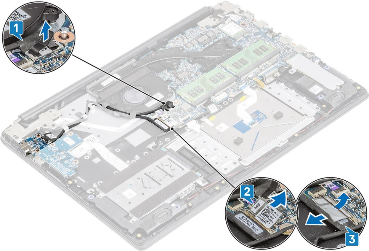
2 Unroute the VGA board cable and the display cable from the routing guides on the fan.
