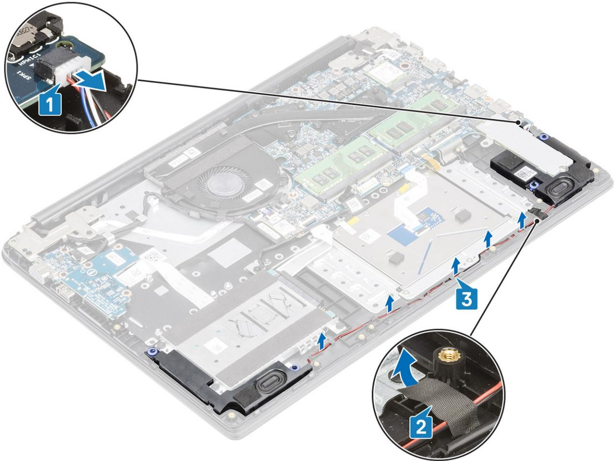
4 Lift the speakers, along with the cable, off the palm rest and keyboard assembly.
