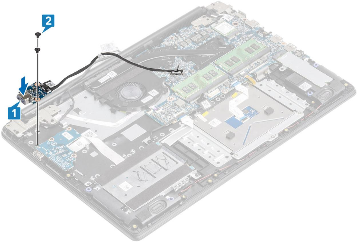
3 Route the VGA board cable and the display cable through the routing guides on the fan.
