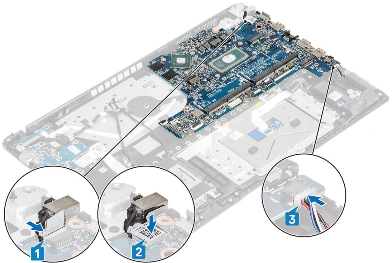
4 Connect the following cables to the system board:
