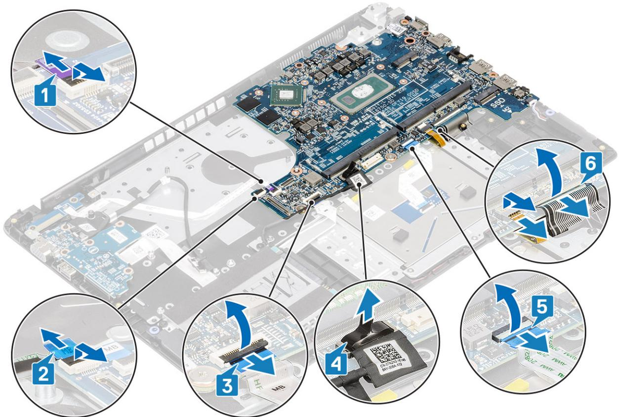
2 Disconnect the following cables from the system board:
