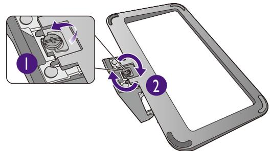
Orient and align the stand arm with the monitor, then push them together until they click and lock into place.
