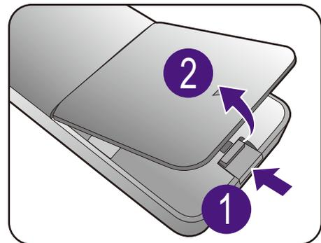
2. Press down the upper part of the battery so you can remove the battery from the lower part as illustrated.
