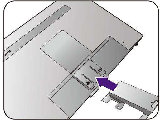
Tighten the screws that fix the stand to the monitor.
