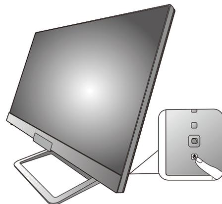
Turn on the computer too, and press the 5-way controller to select an input source. The displayed input icons vary depending on the available video inputs of the purchased model.
