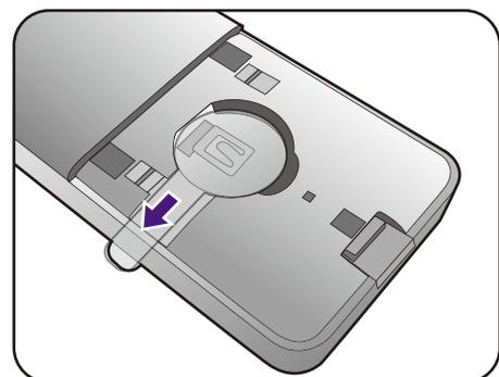
4. Replace the provided battery (CR2032) onto the battery holder properly. Make sure that the positive terminal (+) faces upward.
