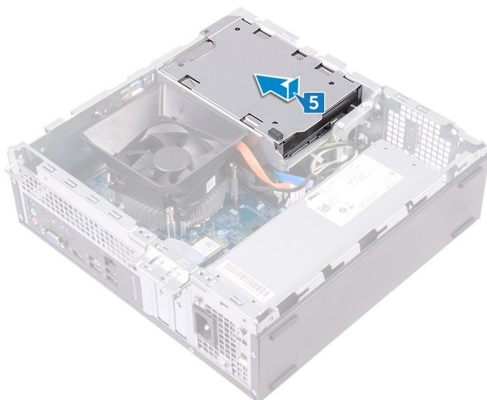
6. Replace the two screws (#6-32x6.35) that secure the hard-drive assembly to the drive cage.
