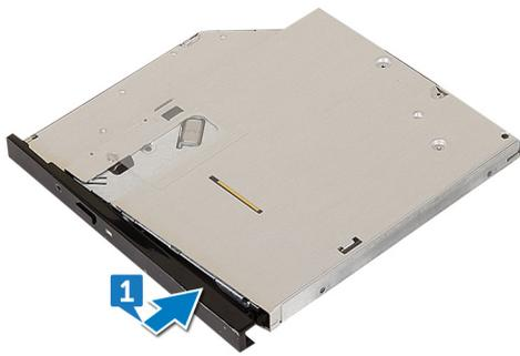
2. Slide the optical drive into the optical-drive cage
