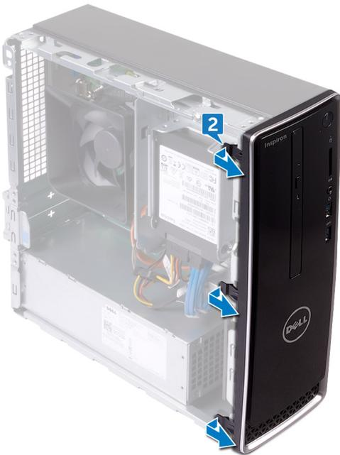
3. Move the front bezel outward from the chassis.
