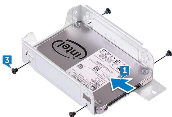
4. Align the screw holes on the top hard drive with the screw holes on the hard-drive bracket.
