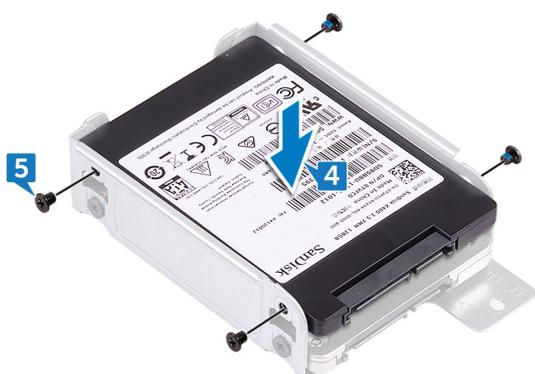
6. Slide the hard drive into the slot on the drive cage until it snaps into place.
