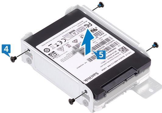
6. Remove the four screws (M3x3.5) that secure the bottom hard drive to the hard-drive bracket.
