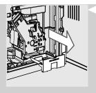
2 Empty and clean the coffee residues drawer located inside of the machine. Open the service door, remove the drawer and empty it.
