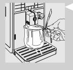
2 Press the "" button to start the cycle. The machine starts the automatic priming of the circuit by dispensing some water through the coffee dispensing spout.
