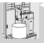
10 Pull the milk carafe dispenser to the left up to the " \_\_\_\_ " icon. Place a large container (1.5 lt) under both the milk carafe dispenser and the dispensing spout.
