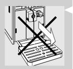
NEVER remove the drip tray when the machine has just been turned on. Wait a couple of minutes for the machine to carry out a rinse/selfcleaning cycle.
