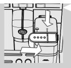
10 Put back the milk carafe dispenser by shifting it up to the "●" icon. Remove the milk carafe and empty it.
