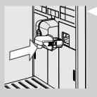
1 Slightly tilt the water dispensing spout and then insert it all the way in into the guides of the machine.
