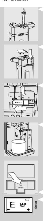
4 Remove the lid and fill the milk carafe up to the MAX level with fresh water.
