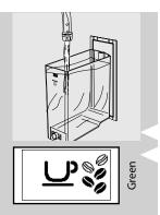
14 At the end, fill the water tank again up to the MAX level. Now the machine is ready for brewing coffee.
