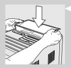
4 Insert the coffee bean hopper into the compartment as shown on the image.
