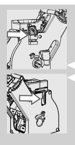
10 Make sure the hook to lock the brew group is in the correct position by firmly pressing the "PUSH" button until it locks into place. Check if the hook is at the top end position. If it is not, please try again.
