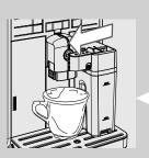
Each time the "" button is pressed, the machine pours a pre-set quantity of cappuccino into the cup.
