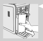
6 Remove the water tank by pulling the handgrip.
