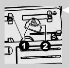
3 The reference marks in the compartment for the coffee bean hopper indicate the grind setting. There are 5 different grind settings to choose from position1 for coarse grind - lighter taste to position 2 for fine grind - bolder taste.
