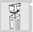
3 Attach the top on the milk carafe; ensure it is locked into place.
