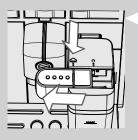
3 Insert the carafe into the machine. Pull the milk carafe dispenser to the left up to the " \_\_\_\_ "icon.
