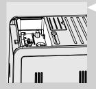
To remove the tray push the hooks on the bottom of the coffee bean hopper. This is shown in the picture on the left.
