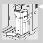
3 Push the carafe towards the bottom while rotating at the same time, until it is locked at the drip tray.
