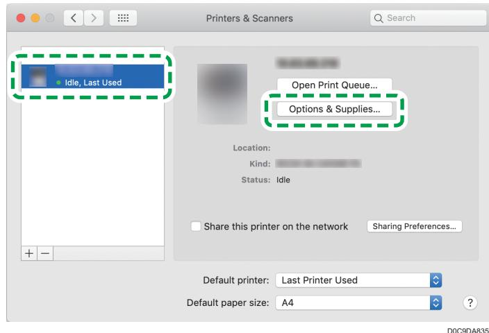
**4. Click [Driver] or [Options], select the option installed on the machine, and then click [OK].**
