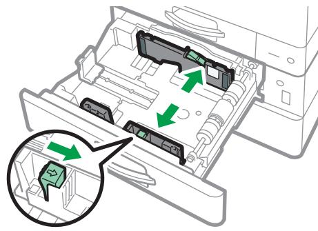
**5. While pinching the release lever of the end fence, slide the end fence outward.**
