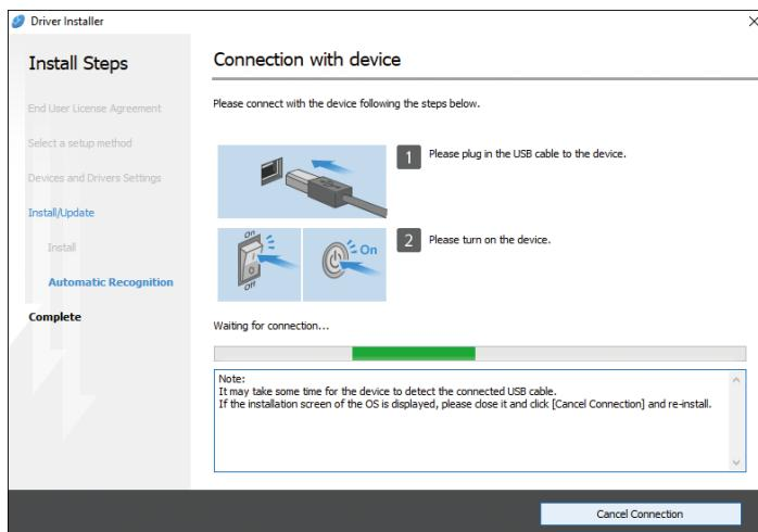
If the machine is not detected, click [Cancel Connection]. Even if the connection is canceled, the installation is complete. After the installer screen is closed, the machine is added automatically when it is connected to the computer with the USB cable.
