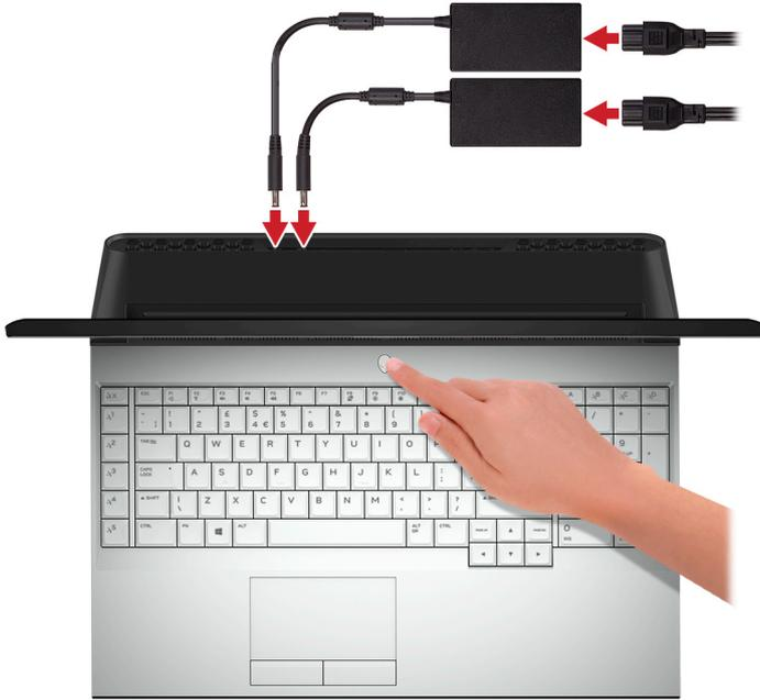
**NOTE:** Your computer ships with two power adaptors, and it will operate normally with one power adapter connected. For maximum gaming performance, it is recommended to connect two adapters. Only use adapters supplied with your device, or Dell-approved adapters to power your device.
