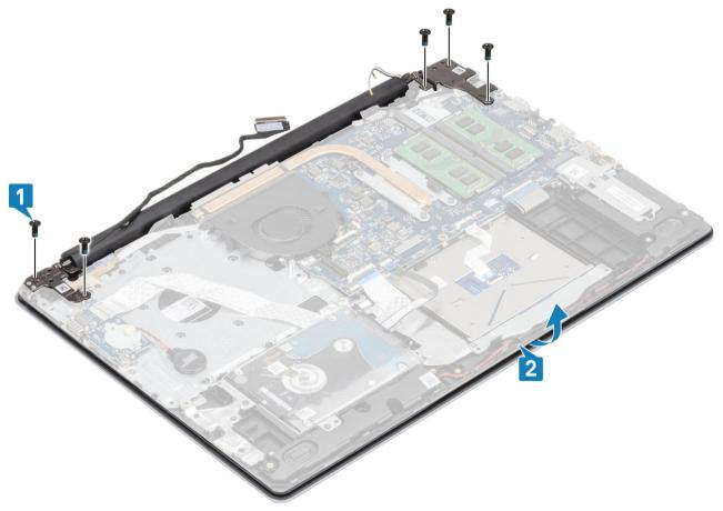
6 Lift the hinges and remove the palmrest and keyboard assembly off the display assembly [1, 2].
