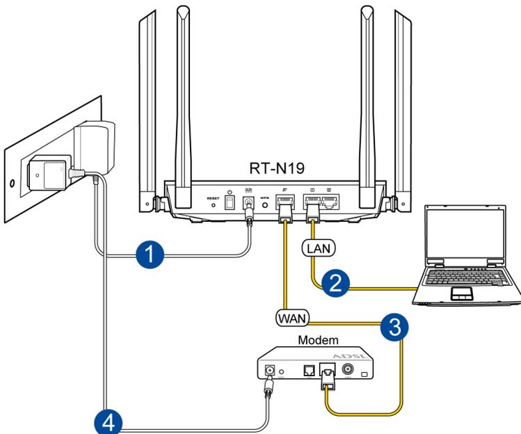
**To set up your wireless router via wired connection:**
