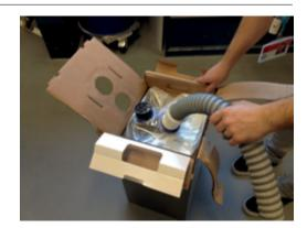
7. Switch-on the explosionprotected vacuum cleaner to remove the air from the bag while pushing it downwards to separate the plastic bag from the cardboard.
