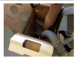
8. Take out the collapsed bag and remove the connector from the explosion-protected vacuum cleaner.
