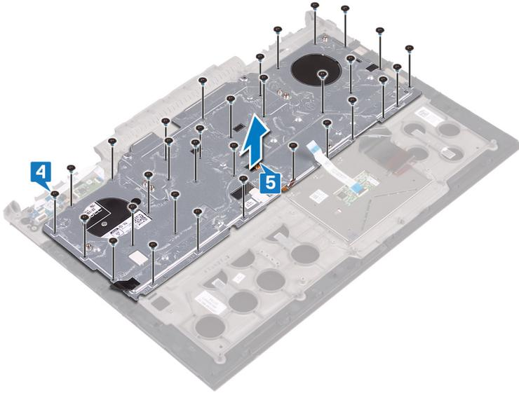
6 Lift the keyboard, along with the cables, off the palm-rest assembly.
