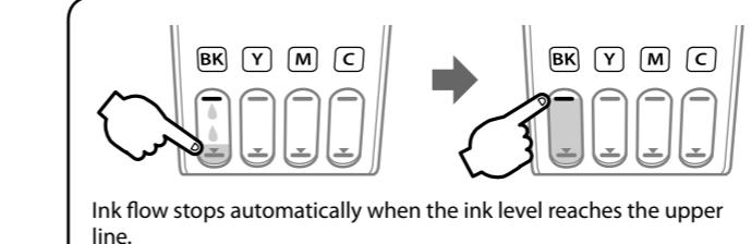
Ink flow stops automatically when the ink level reaches the upper line.
