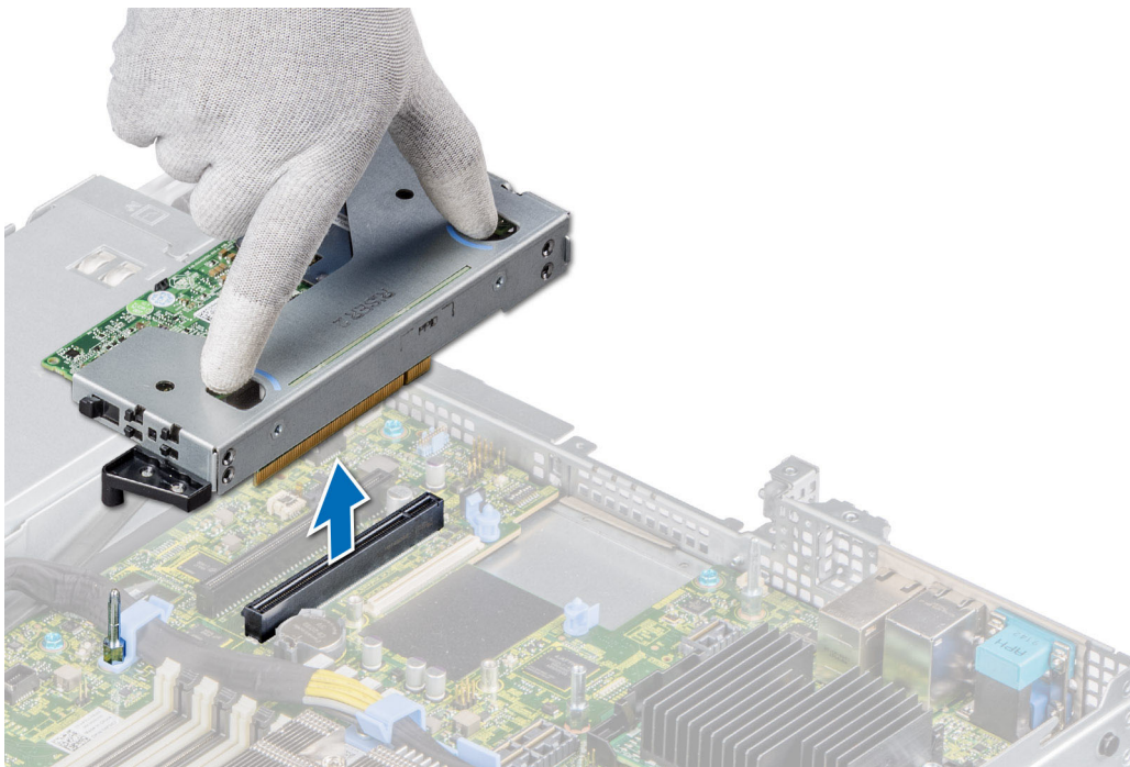
Figure 54. Removing the low profile left riser
