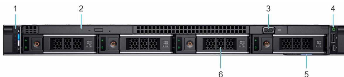
Figure 1. Front view of 4 x 3.5-inch drive system
