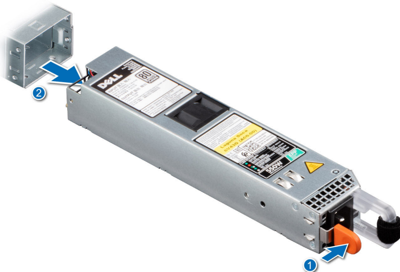
Figure 92. Removing a power supply unit
