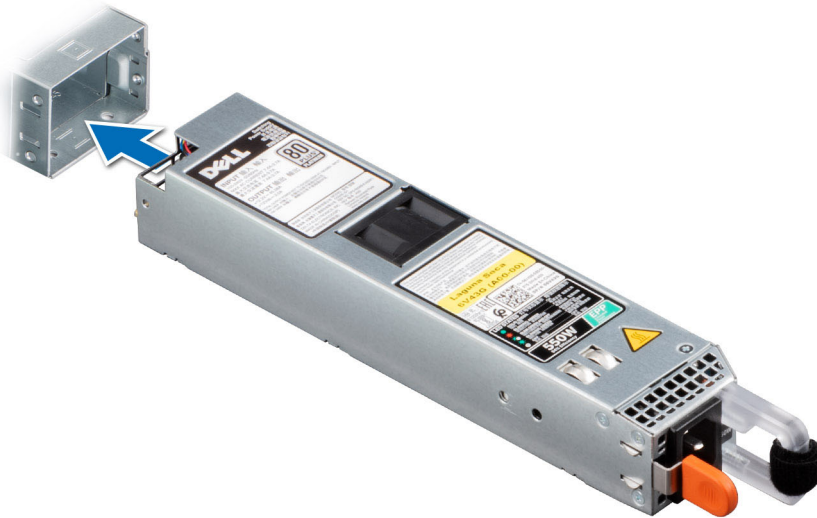
Figure 93. Installing a power supply unit
