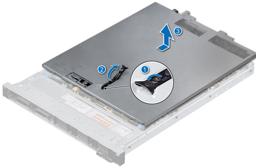
Figure 17. Removing the system cover
