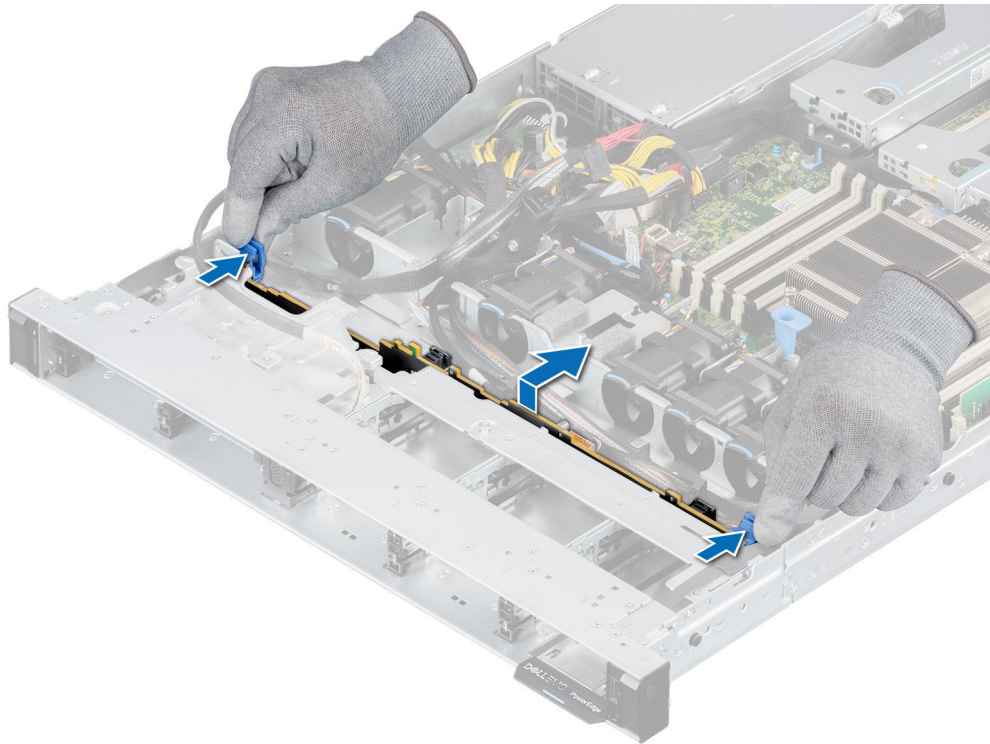
Figure 36. Removing the backplane
