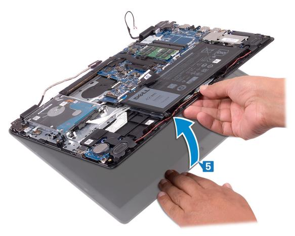
6 Slide and remove the palm-rest and keyboard assembly off the display assembly.
