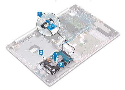
4. Disconnect the interposer from the hard-drive assembly.
