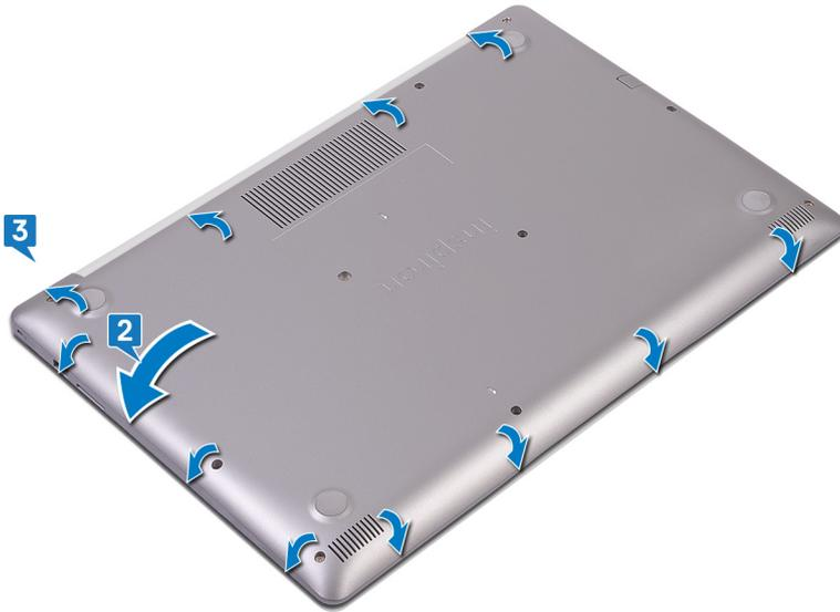
4. Tighten the three captive screws that secure the base cover to the palm-rest and keyboard assembly.
