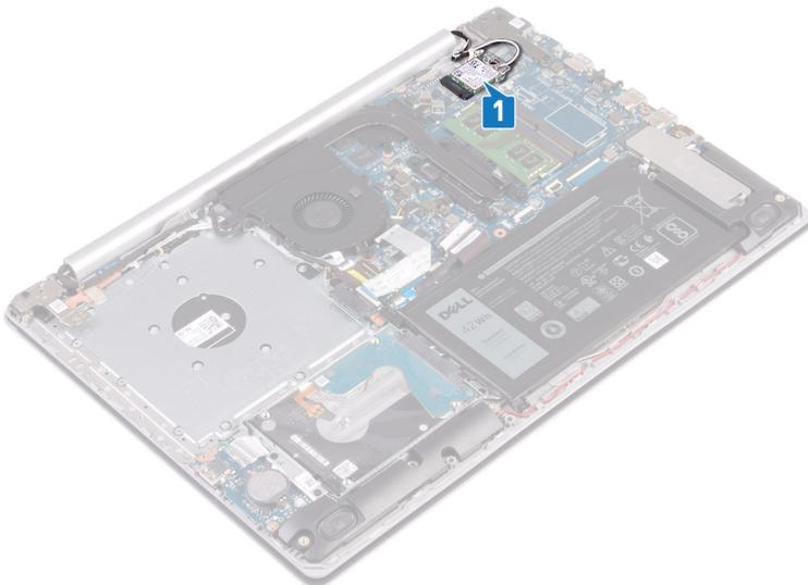
2. Remove the screw (M2x3) that secures the wireless-card bracket to the system board.
