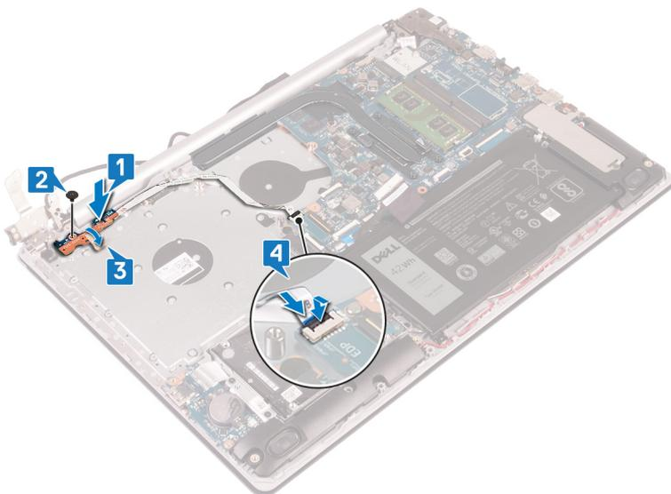
5. Route the display cable through the hook on the right hinge and close the right hinge.
