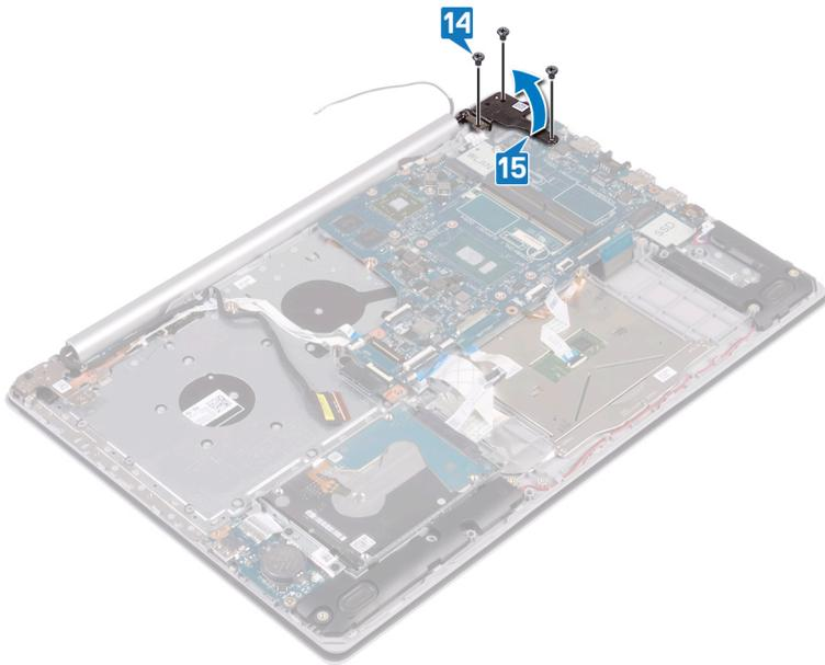
16. Remove the screw (M2x4) that secures the system board to palm rest and keyboard assembly.
