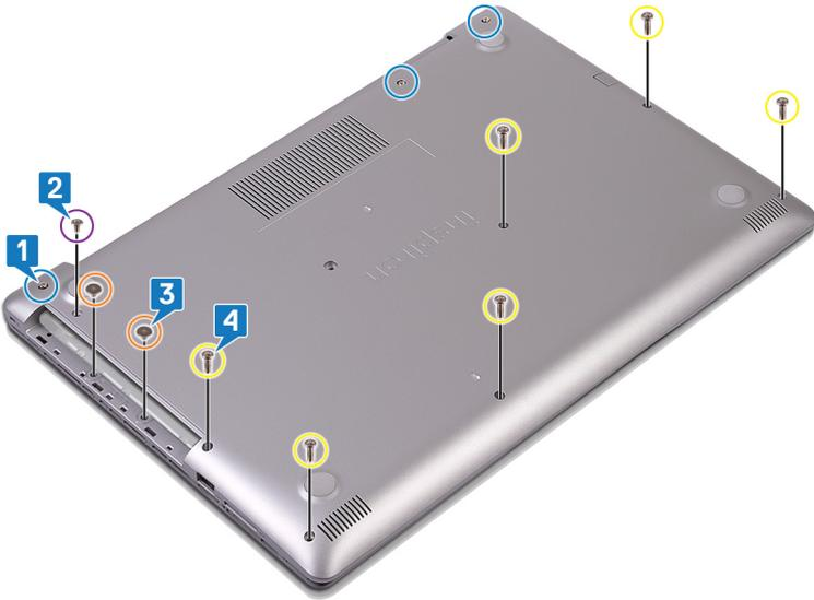
5. Pry the base cover starting from the top-left corner of the computer base.
