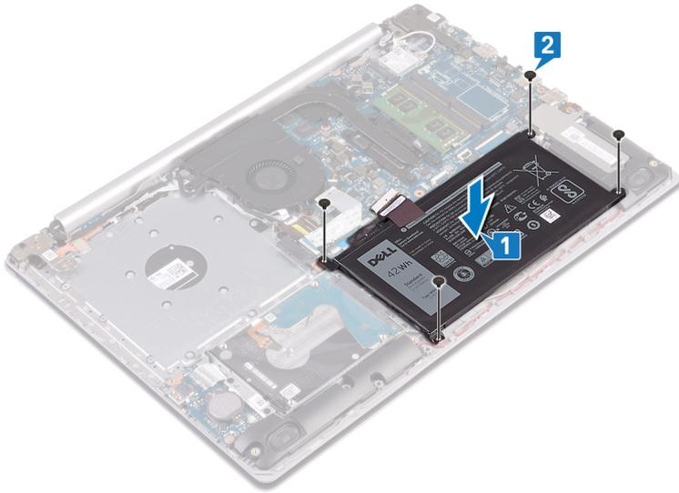
3. Connect the battery cable to the system board.
