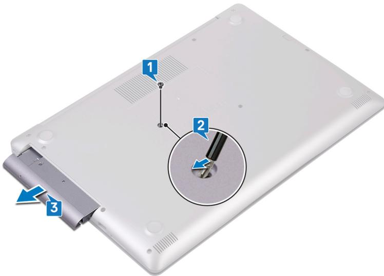
4. Remove the two screws (M2x3) that secure the optical-drive bracket to the optical drive.
