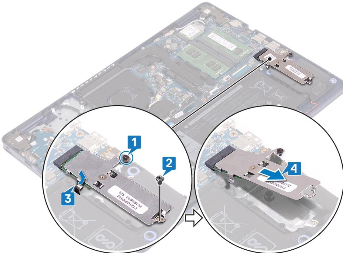
5. Turn the M.2 2230 thermal shield over.
