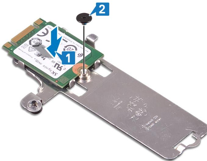
3. Turn over the solid-state drive and M.2 2230 thermal shield.
