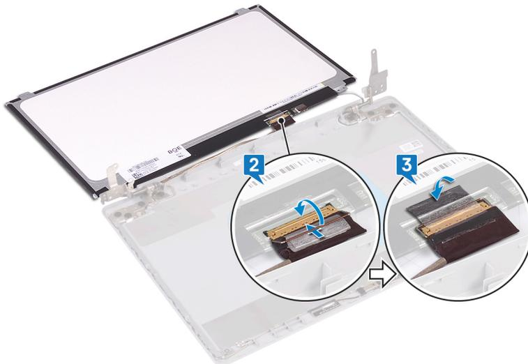
4. Place the display panel on the display back-cover and antenna assembly.
