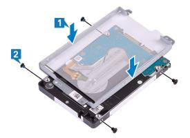
3. Connect the interposer to the hard-drive assembly.
