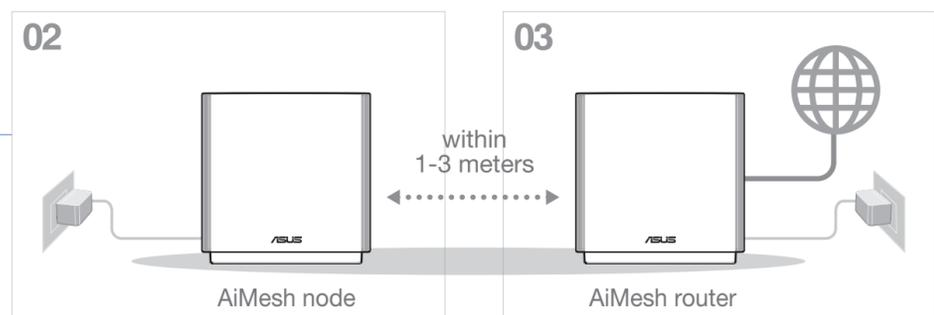
**NOTE:** When you're using a wireless backhaul to connect your router and AiMesh node, the WAN port on your AiMesh node can be used as a LAN port providing up to 2.5G transmission speed.
