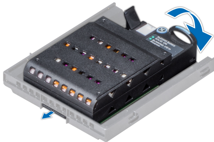
Figure 45. Installing NVDIMM-N battery into the bracket
