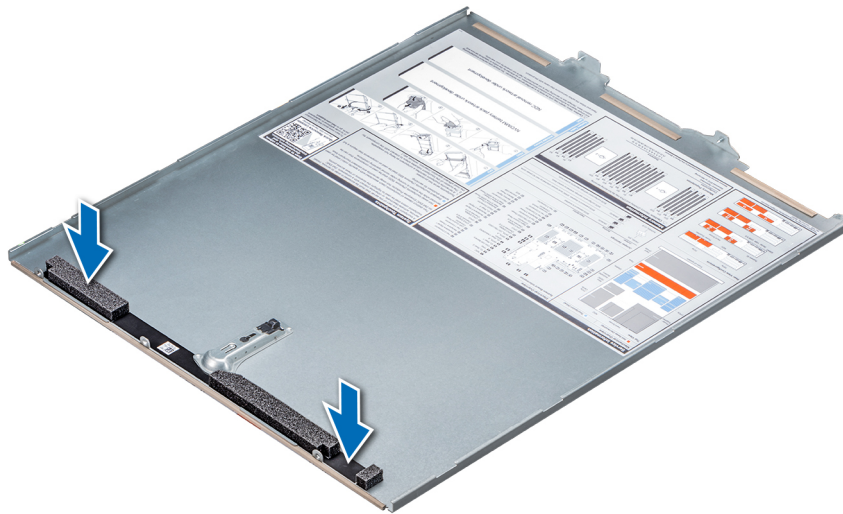
Figure 98. Installing mylar foam on the system cover
