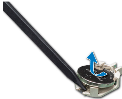
Figure 121. Removing the system battery
