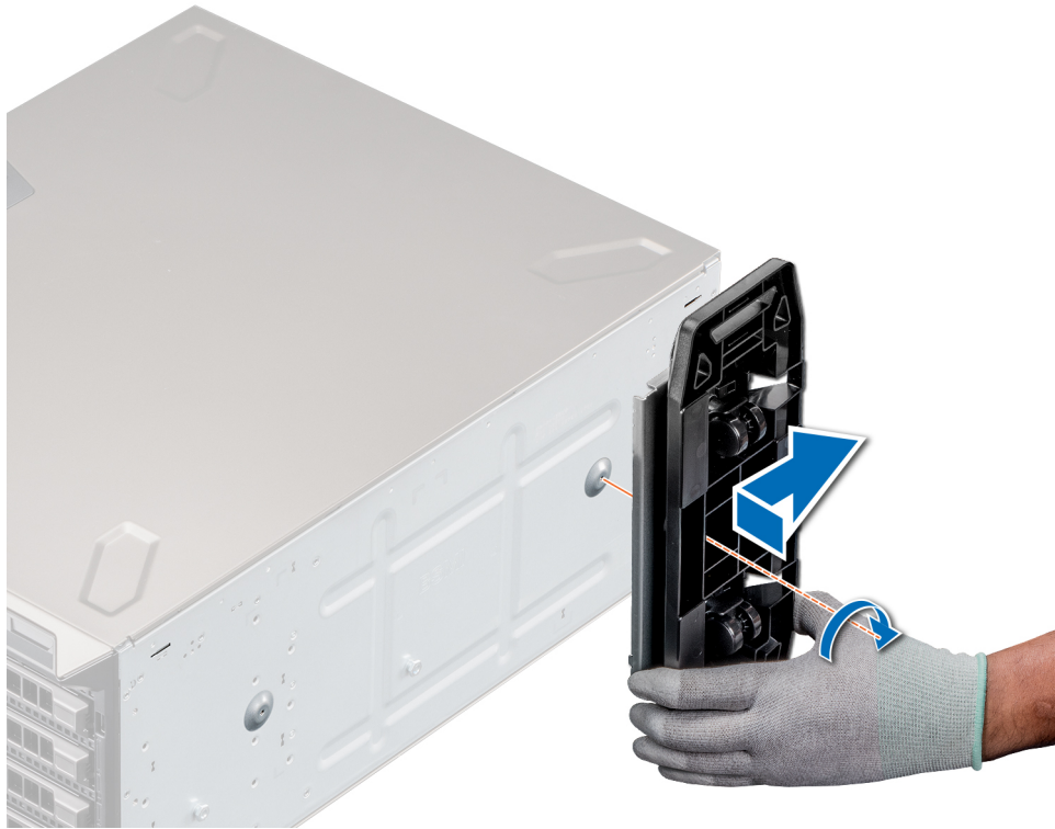
Figure 21. Installing caster wheels
