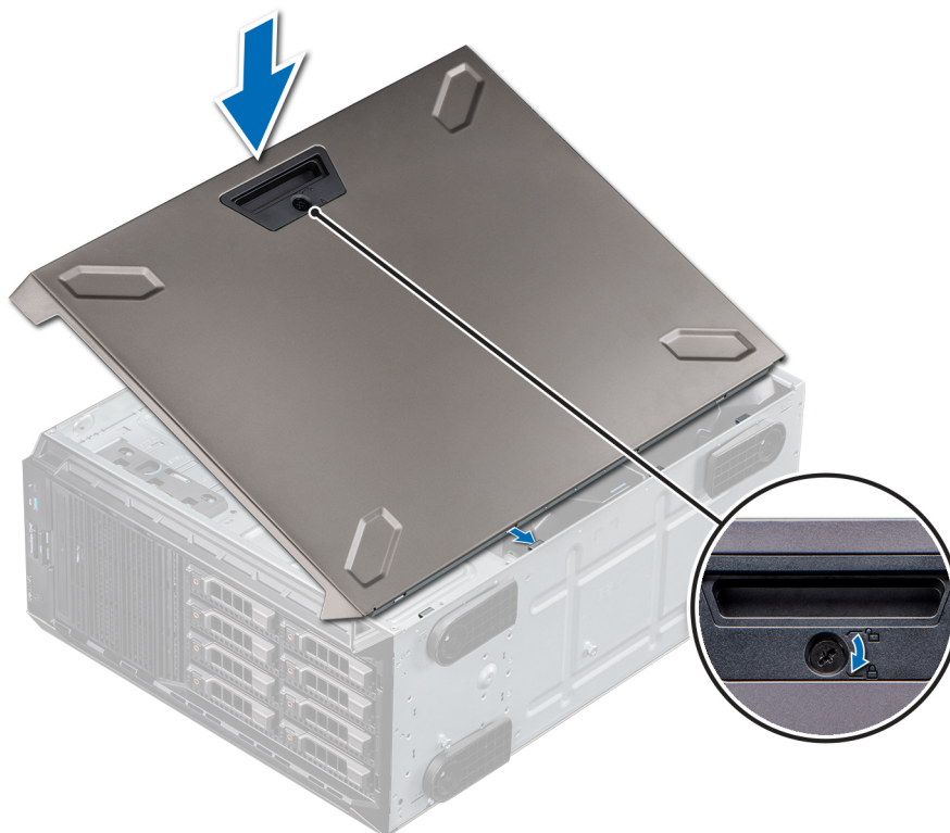
Figure 23. Installing the system cover
