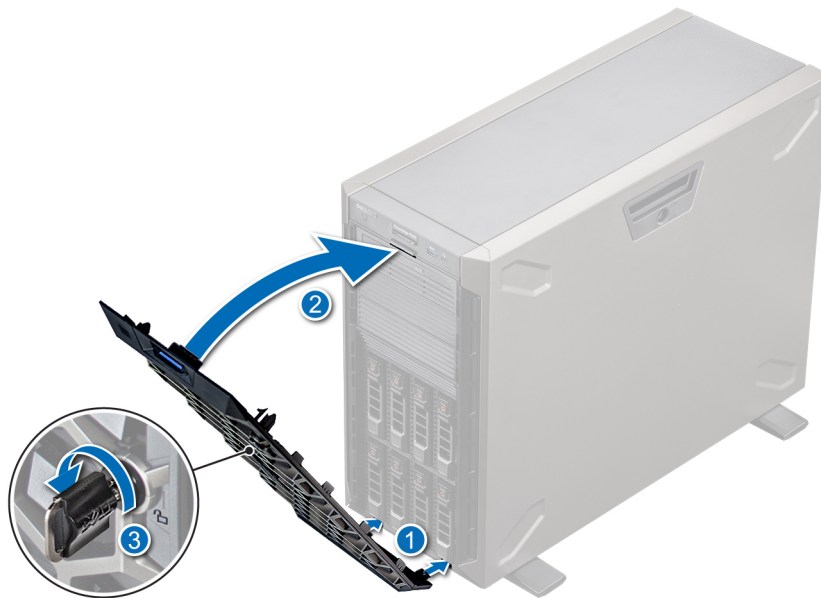
Figure 18. Installing the front bezel
