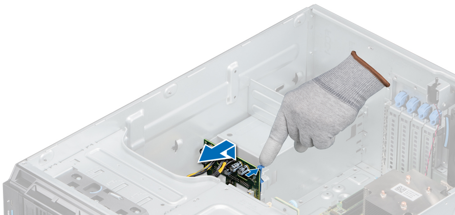
Figure 76. Removing the power interposer board
