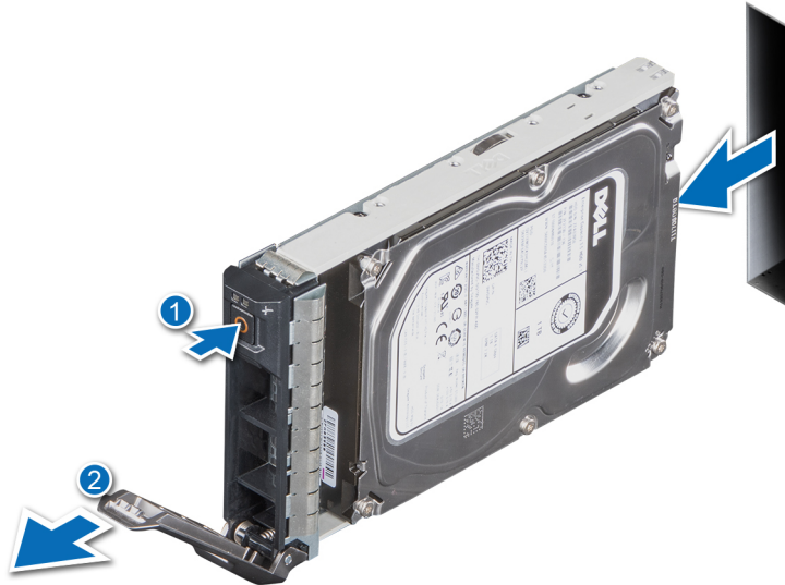
Figure 30. Removing a drive carrier
