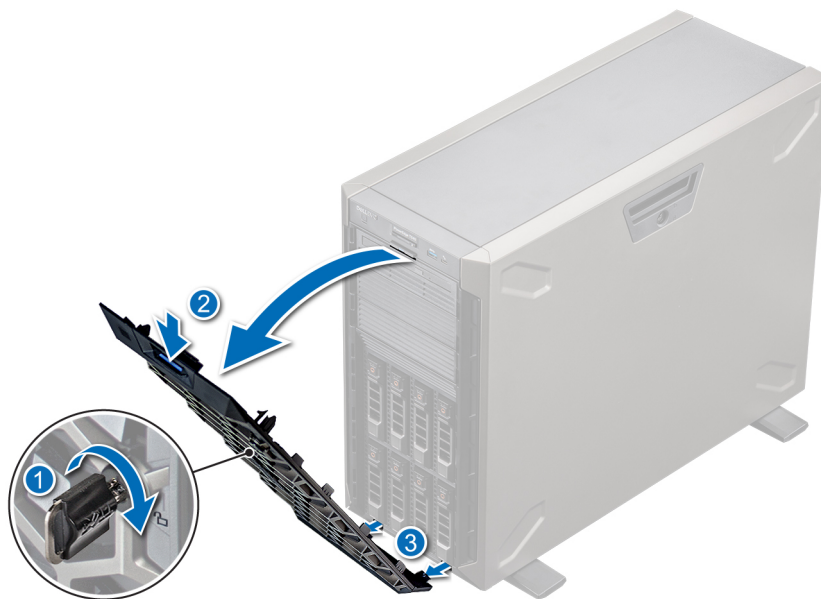
Figure 17. Removing the front bezel
