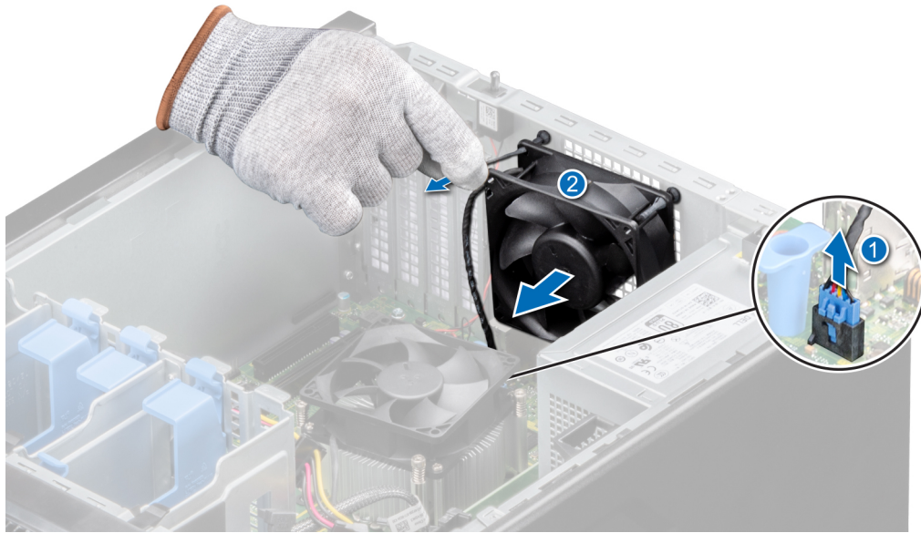
Figure 26. Removing the cooling fan
