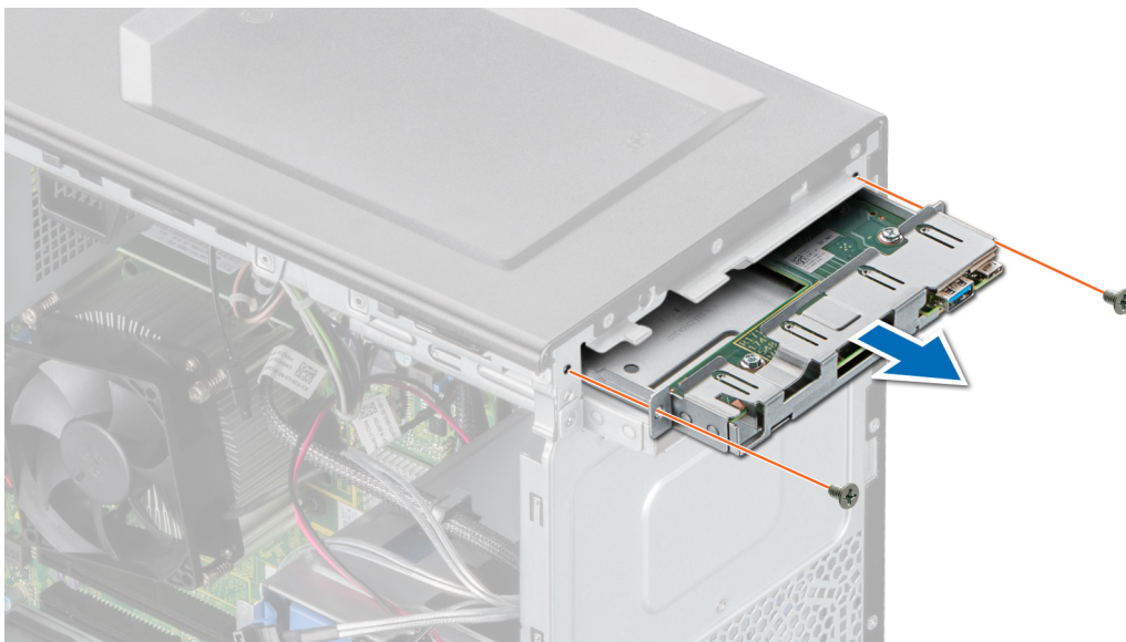
Figure 54. Removing the control panel cage
