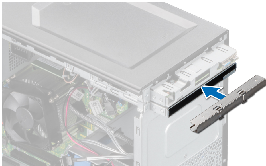
Figure 20. Installing the optical drive filler into the optical drive cage
