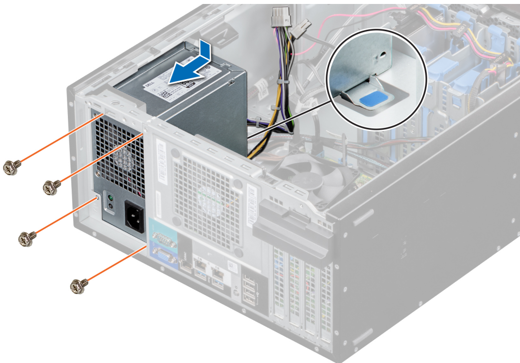
Figure 45. Installing the PSU
